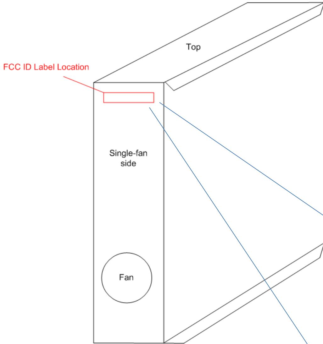
The FCC ID label shall be placed on the single-fan side panel of the chassis. The FCC ID label is approximately 1.4 x 0.3 inches, and the FCC ID is printed in 10pt Arial font.
