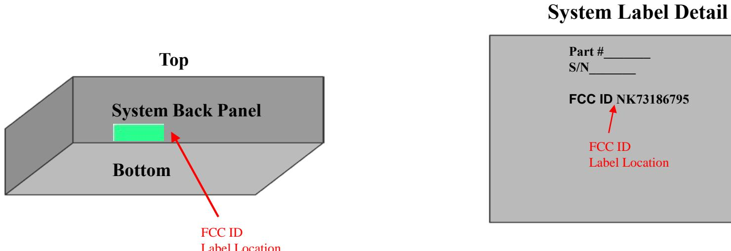
FCC ID label shall be placed on back panel of chassis adjacent to the product part and serial number label. The FCC ID label is approximately 1.4 x 0.3 inches and the FCC ID is printed in 10pt Arial font.
