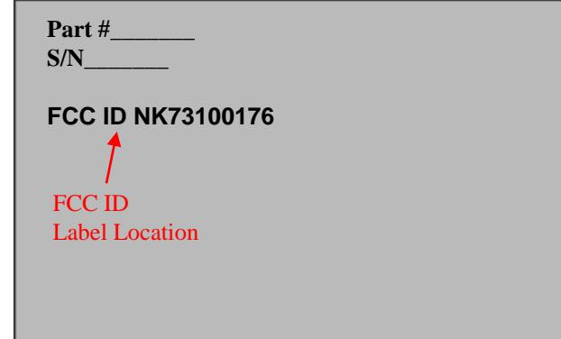
FCC ID label shall be placed on bottom panel of chassis adjacent to the product part and serial number label. The FCC ID label is approximately 1.4 x 0.3 inches and the FCC ID is printed in 10pt Arial font.
