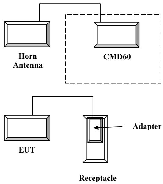
**Block Diagram of Test Setup**
