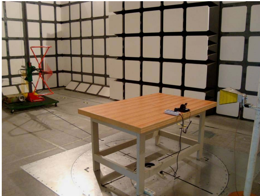
Radiated Emissions - Side View (30 MHz-1000MHz)
