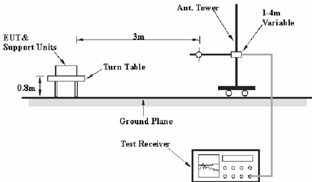
The radiated emission tests were performed in the 3 meters chamber B test site, using the setup accordance with the ANSI C63.17 - 2006. The specification used was the FCC 15.209 and FCC 15.319(g) limits.
