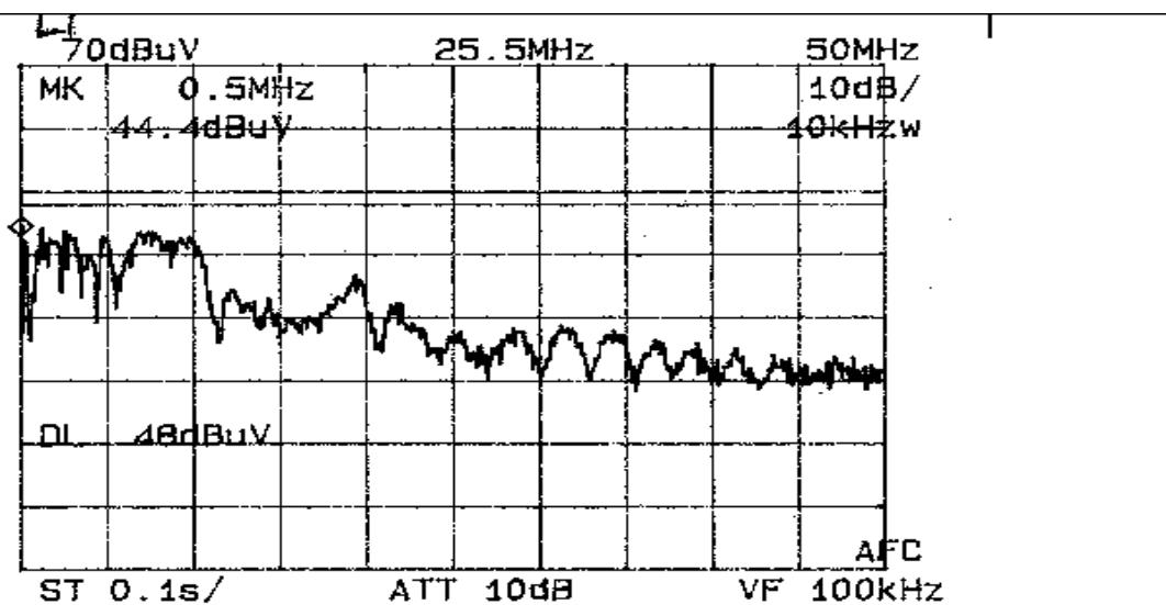
**ioLINK1 A.C. LINE-CONDUCTED EMISSIONS – L2**
