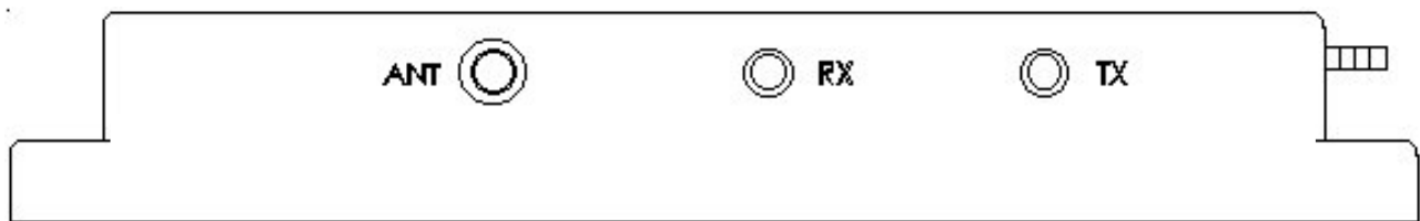
Figure 1-1. View of 5.7-GHz RF Unit Connectors
