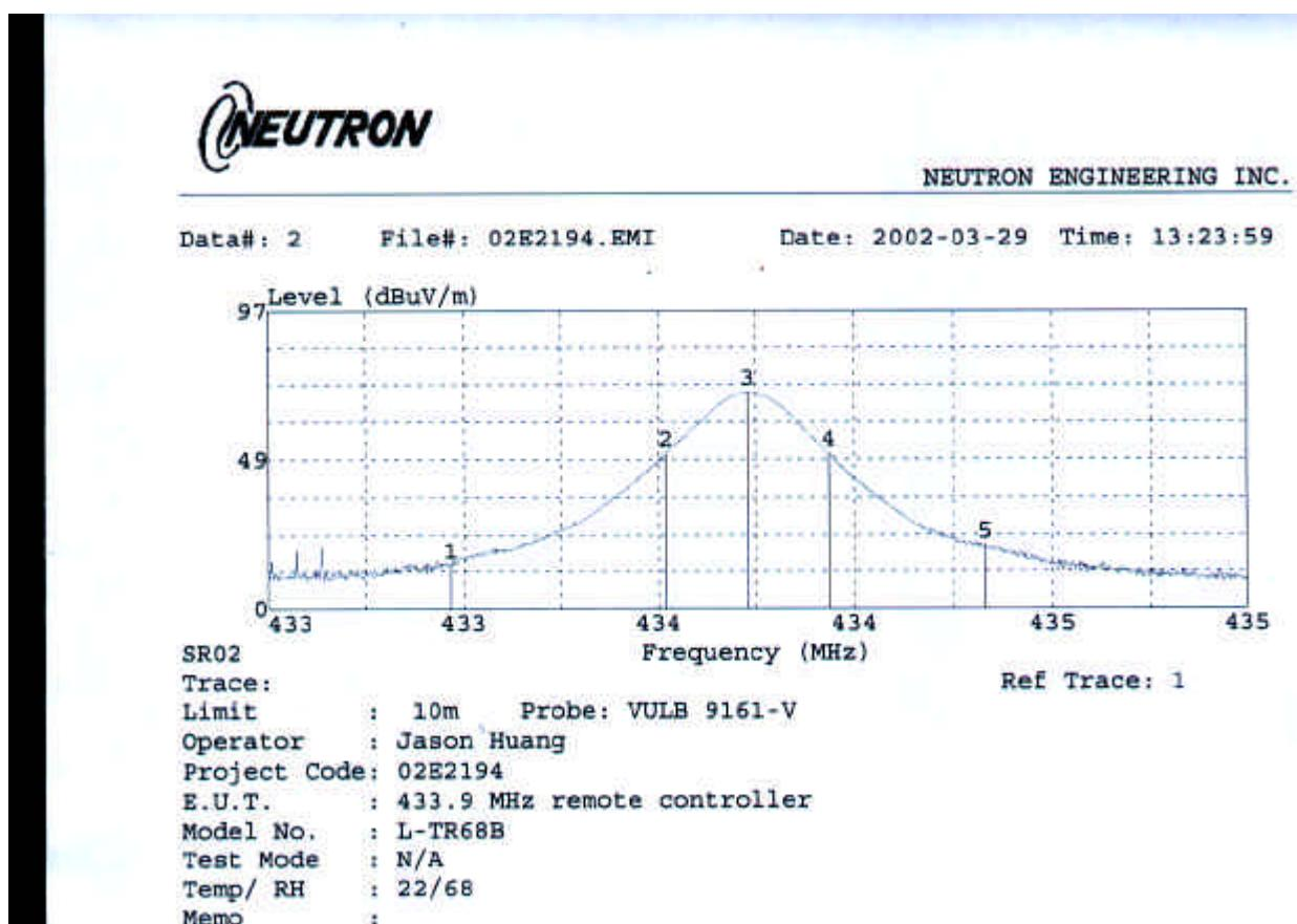
The center frequency  $f_c$  is 433.92MHz (point 3), according to the Rules, section 15.231(C), the Bandwidth
