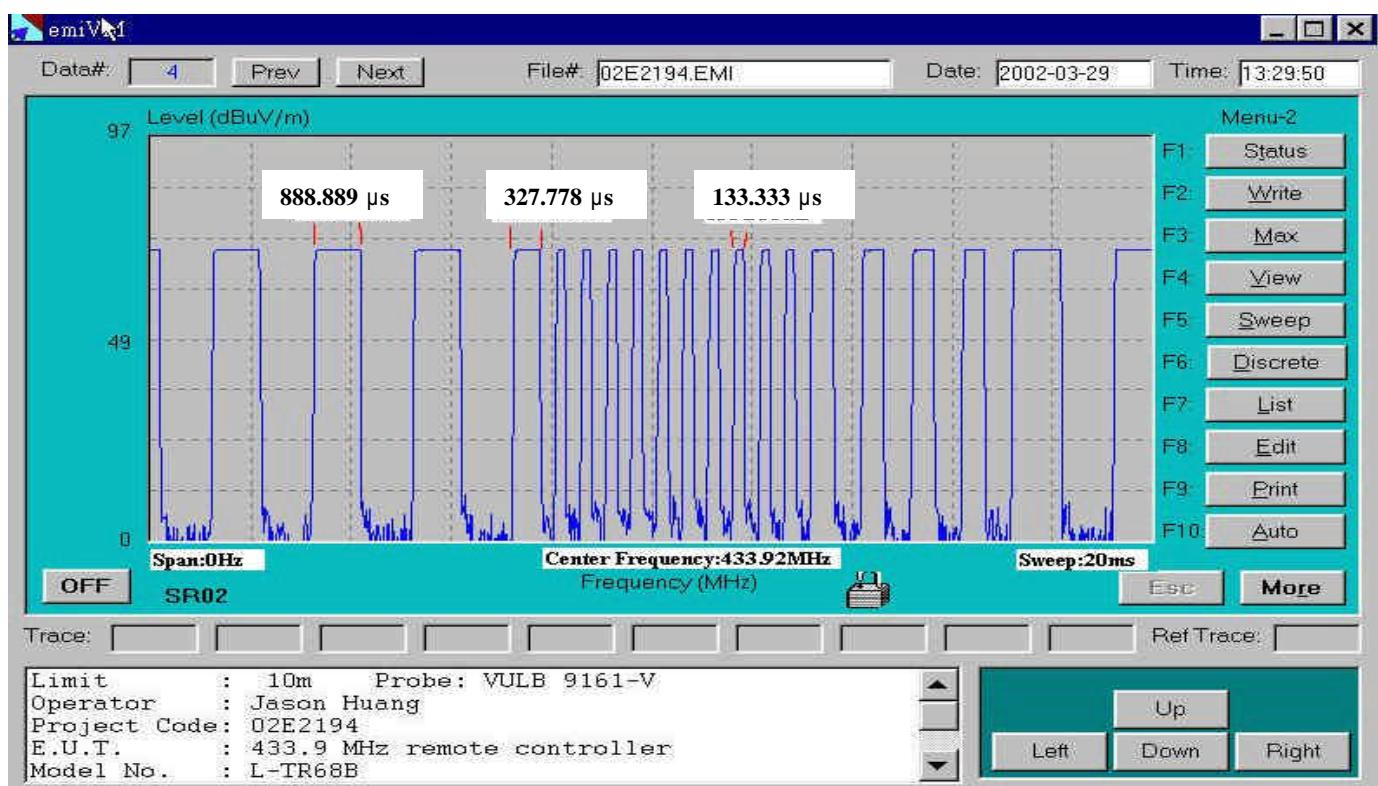
$$Ton = 6 \times 0.889 + 20 \times 0.328 + 25 \times 0.133 \text{ (ms)} = 15.219 \text{ (ms)}$$
