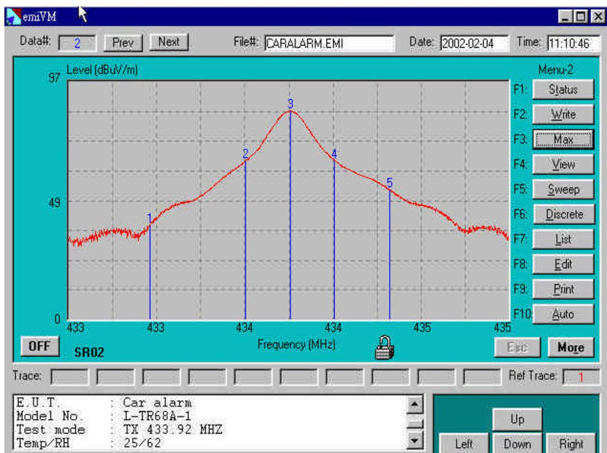
The center frequency **f<sub>c</sub> is 433.92Mhz (point 3)**, according to the Rules, section 15.231(C), the Bandwidth
