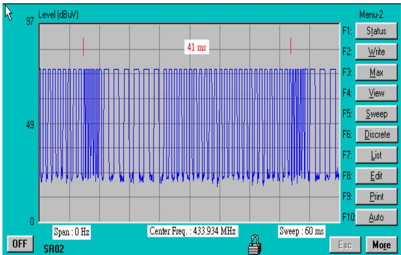
$$T_{on} = 0.2 * 6 + 0.4333 * 26 + 0.9333 * 6 \text{ (ms)} = 18.06 \text{ (ms)}$$
