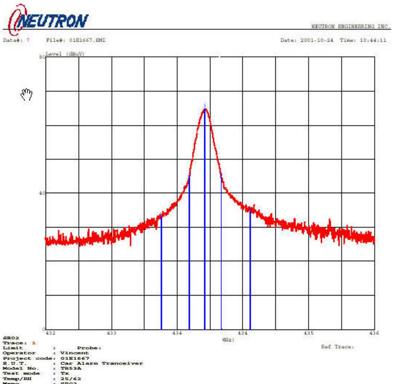
The center frequency **f<sub>c</sub> is 433.92Mhz (point 3)**, according to the Rules, section 15.231(C), the Bandwidth
