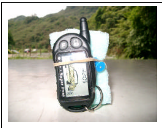
Radiated Open Site Test Set-up (Transmitter Mode)
