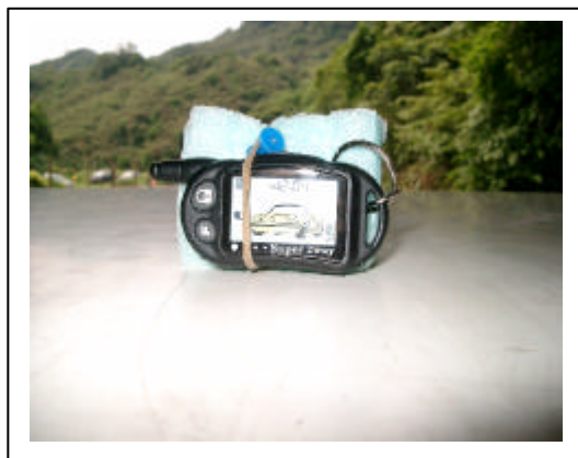
Radiated Open Site Test Set-up (Transmitter Mode)
