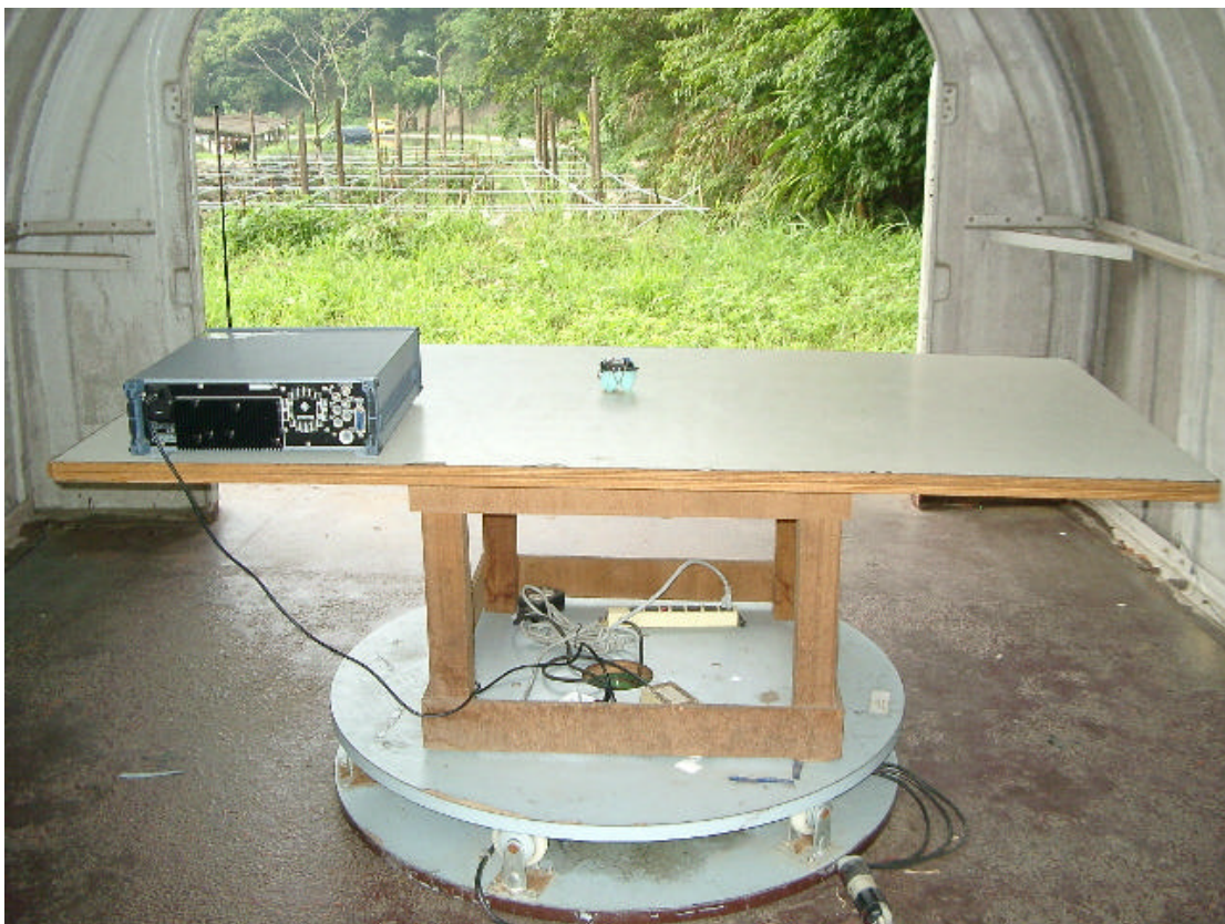
Radiated Open Site Test Set Up (Receiver Mode)
