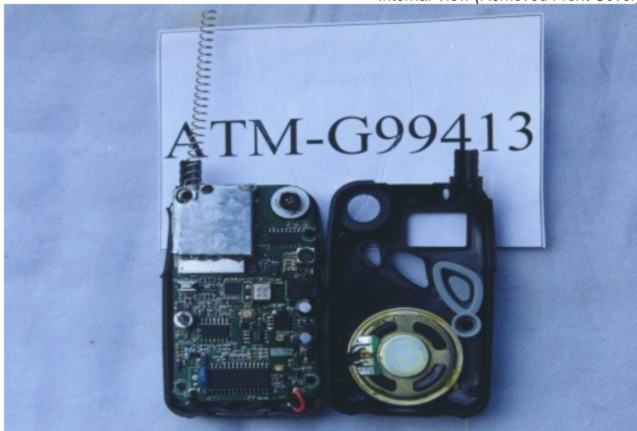
Photo 4 Internal View (Removed Front Cover)
