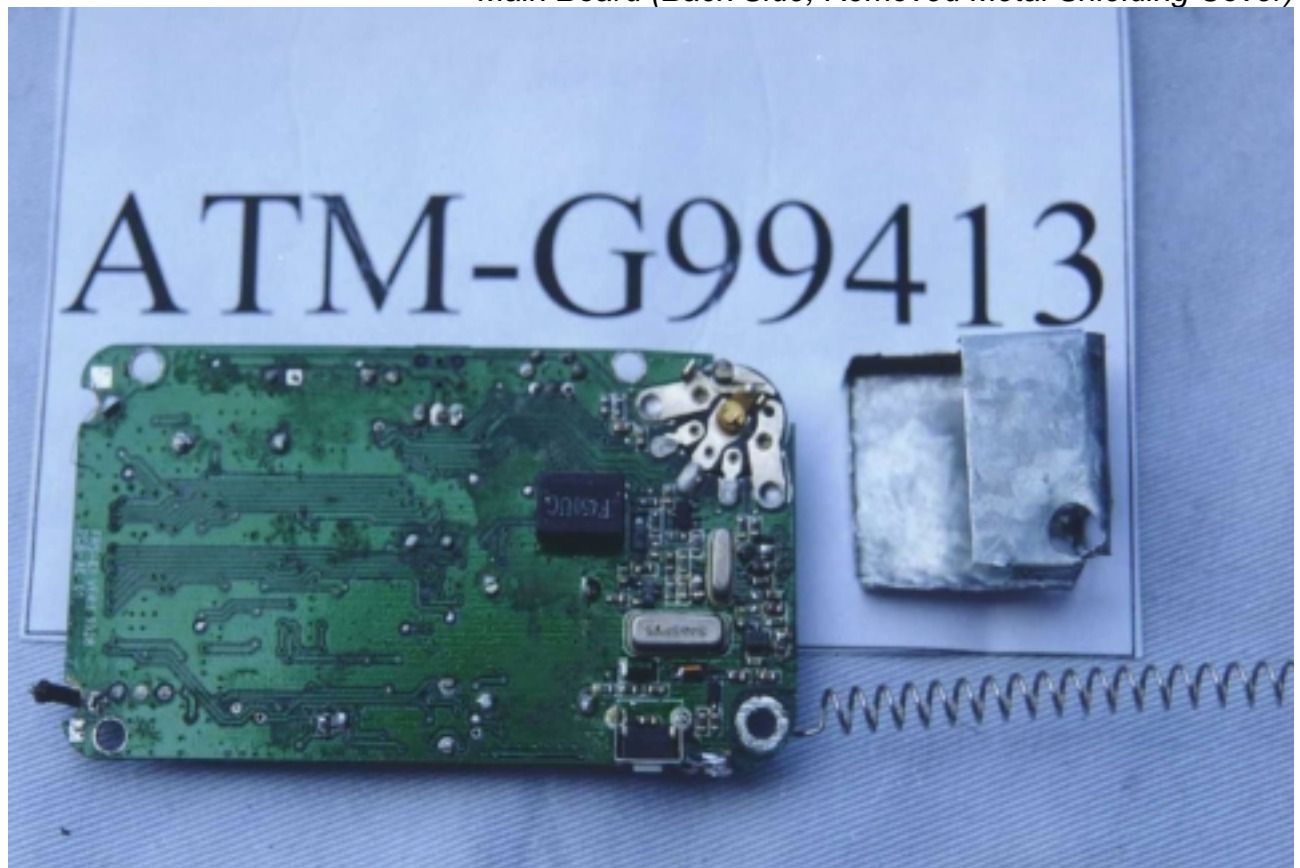
Photo 6 Main Board (Back Side, Removed Metal Shielding Cover)
