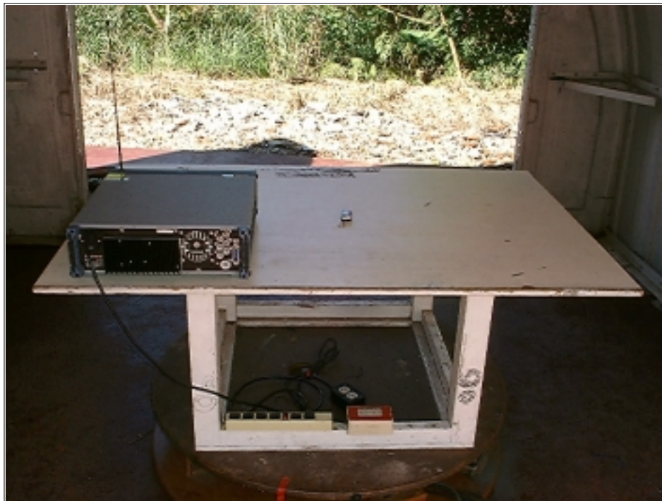
Radiated Open Site Test Set-up (Receiver Mode)
