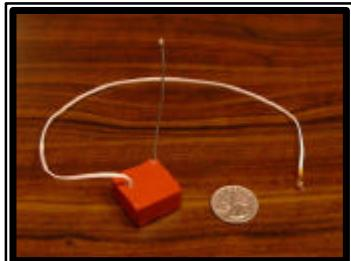
The Sensor Unit can be placed in any location within 100 feet of the PC Interface Unit for reliable operation.
