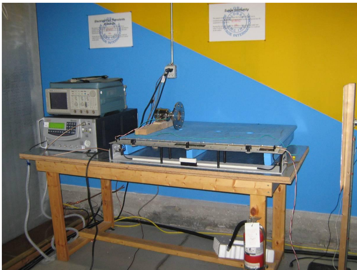
Electronic Fast Transient / Burst Setup – Photo
