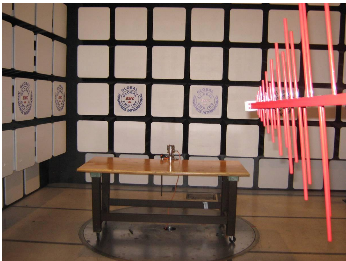
Radiated Emission Setup – Photo 1
