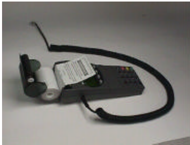
Figure 1: Printer Paper Installation
