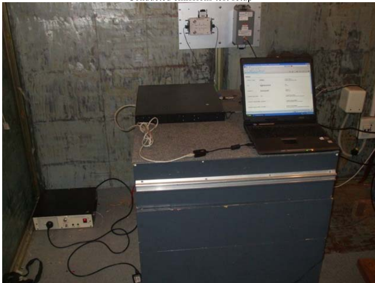
Conducted emissions test setup
