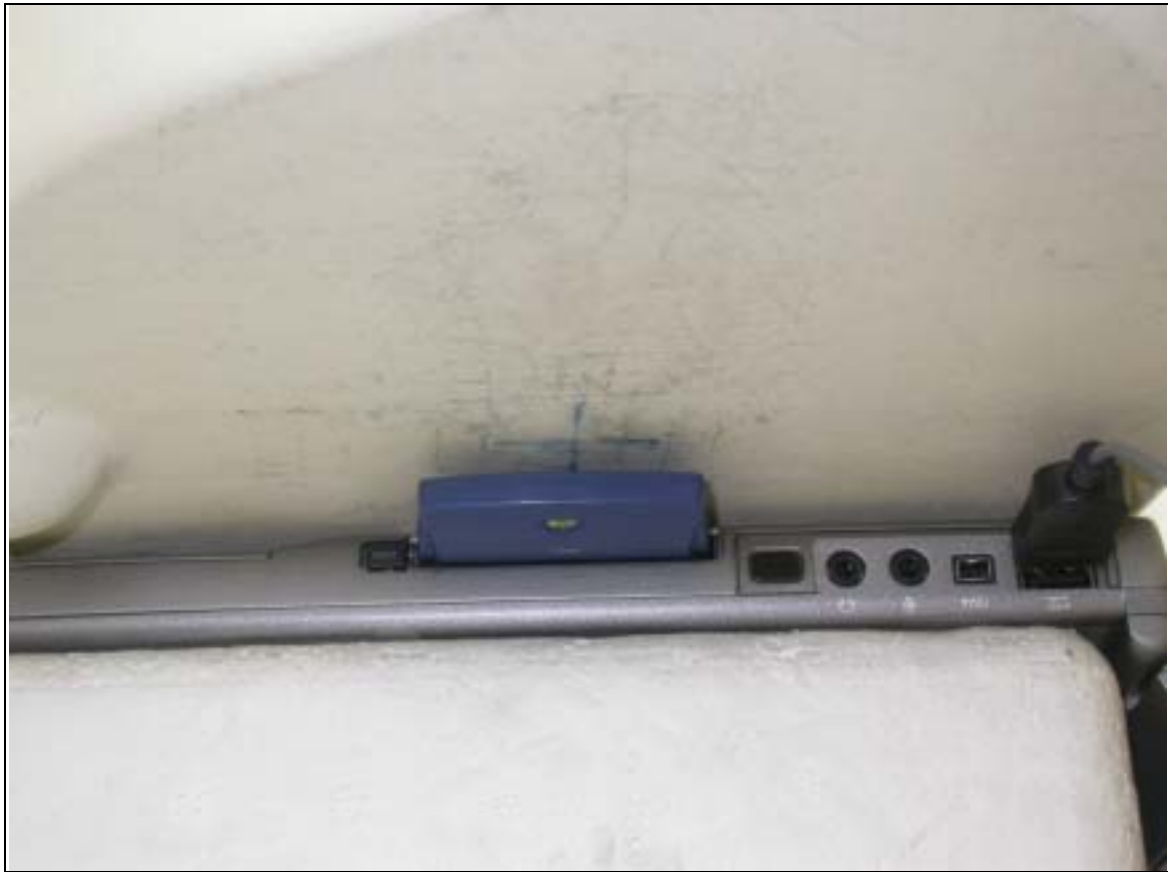
Bottom of the EUT to the flat phantom distance 5mm
