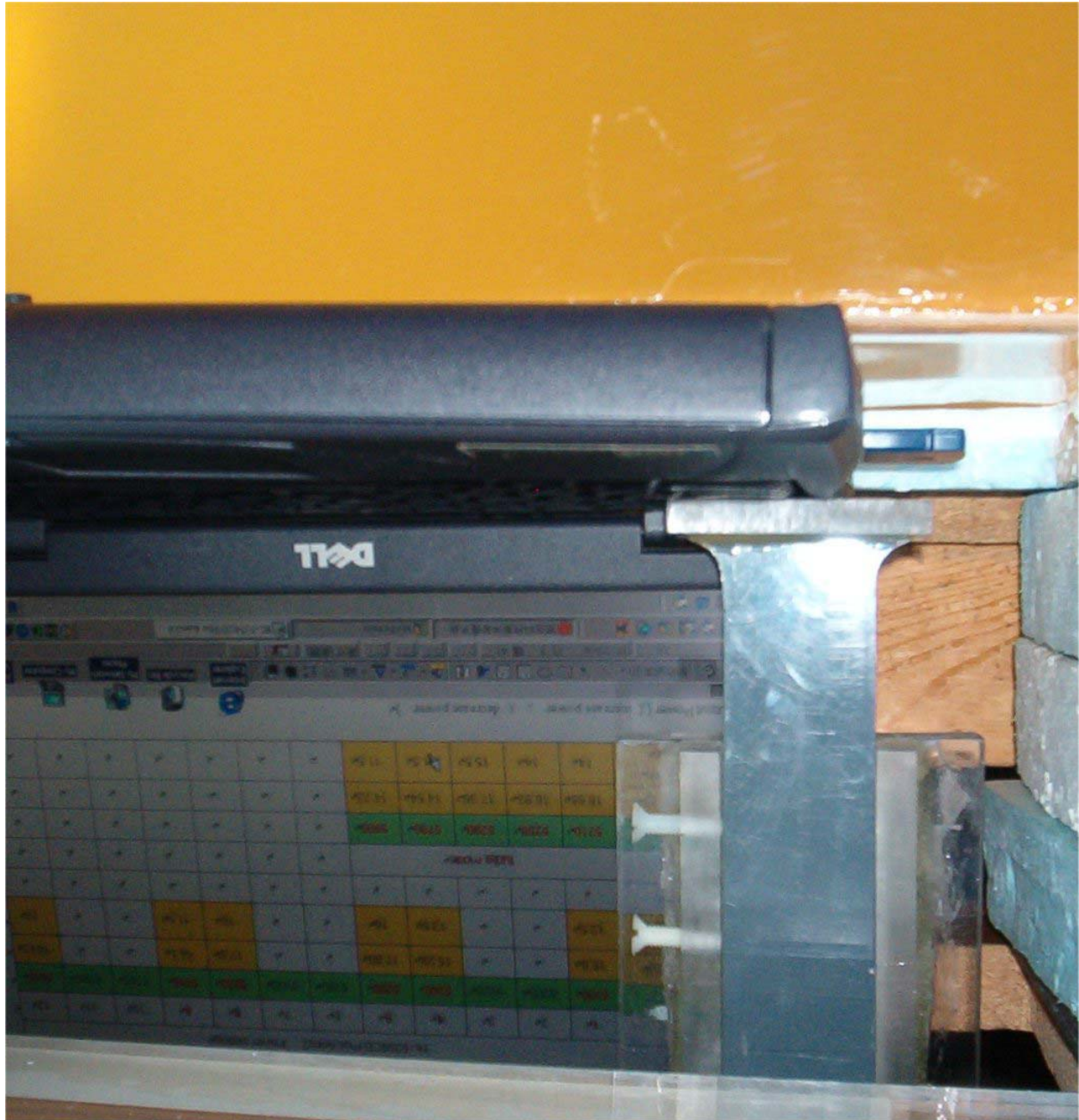
Fig. 2. Photograph of the bottom of the Dell Model PP01L Host Computer with Senao Model NL-5354 CB Plus Aries2 Cardbus Adapter pressed against the bottom of the planar phantom. This Configuration 1 – Laptop position for SAR testing .
