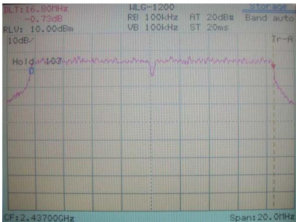
**802.11b Channel 11: 13.16MHz (The minimum 6dB BW at least 500kHz)**
