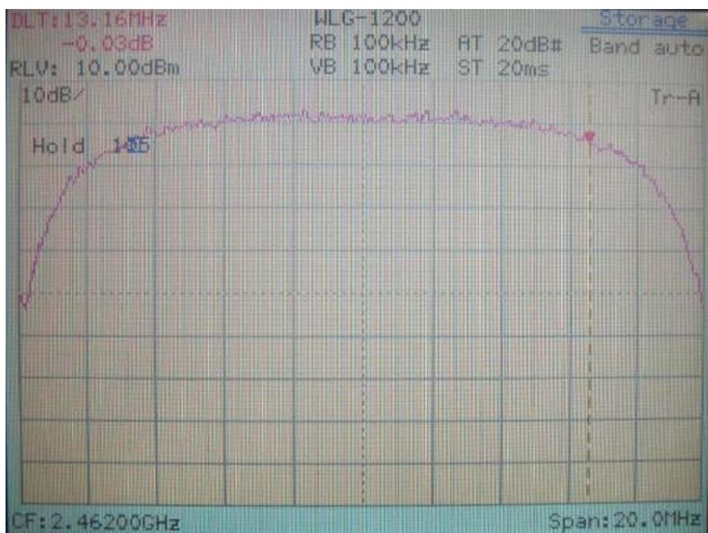
**802.11b Channel 11: 16.88MHz (The minimum 6dB BW at least 500kHz)**
