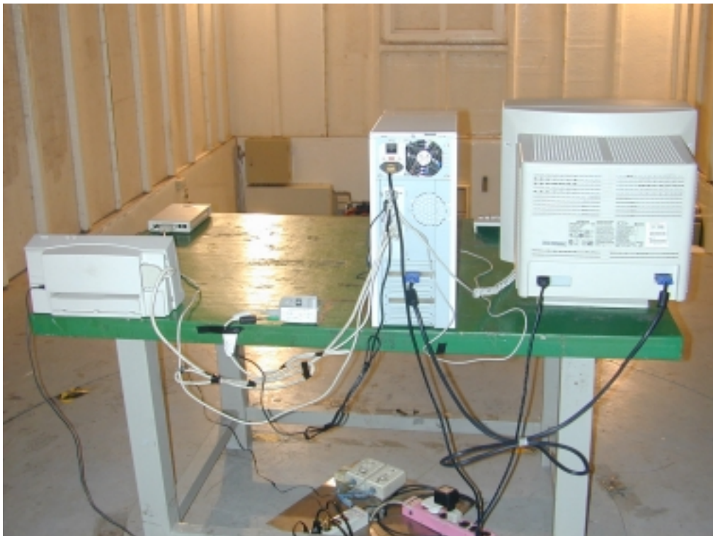
Back View of Radiated Test (Mode 1)
