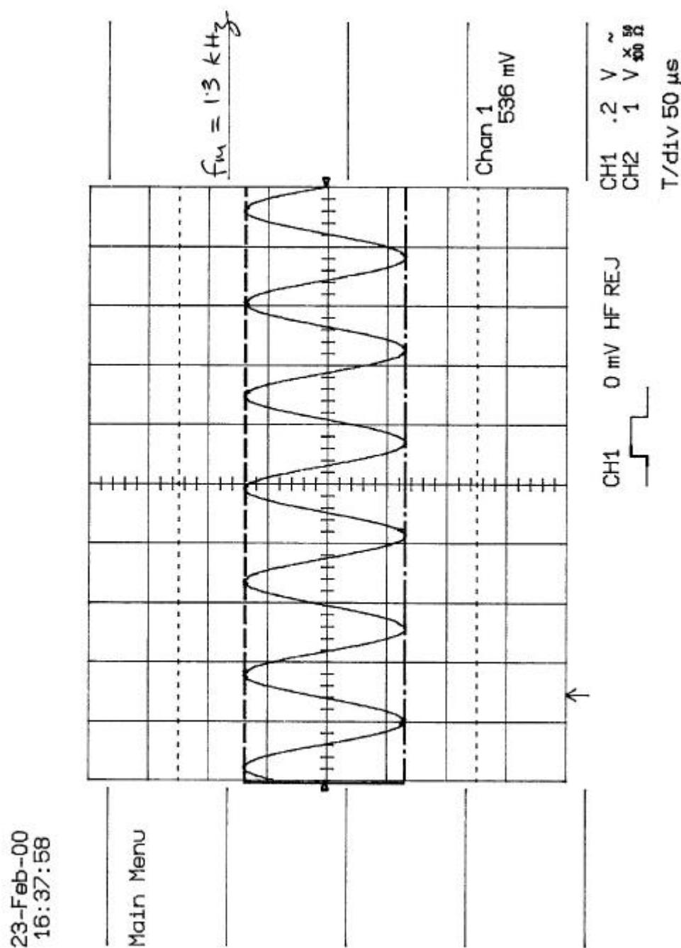
FIGURE 14: Plot of Occupied Bandwidth
