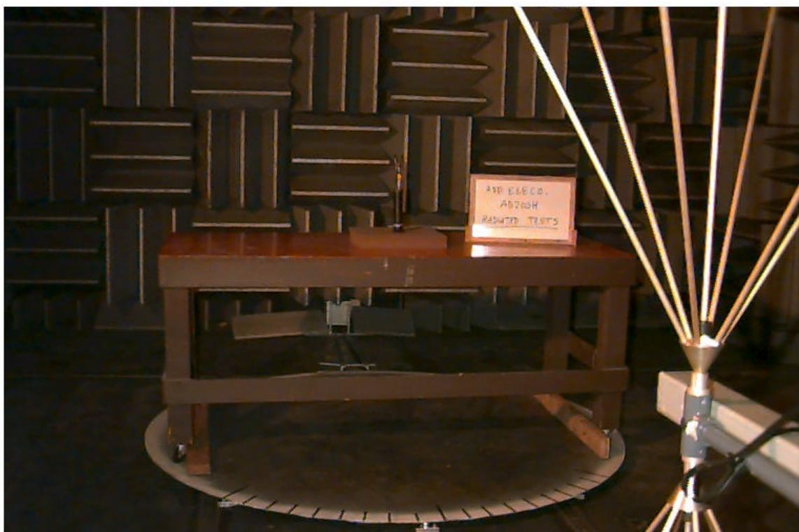
**FIGURE 22: Photograph of Radiated Spurious Emission Setup**
