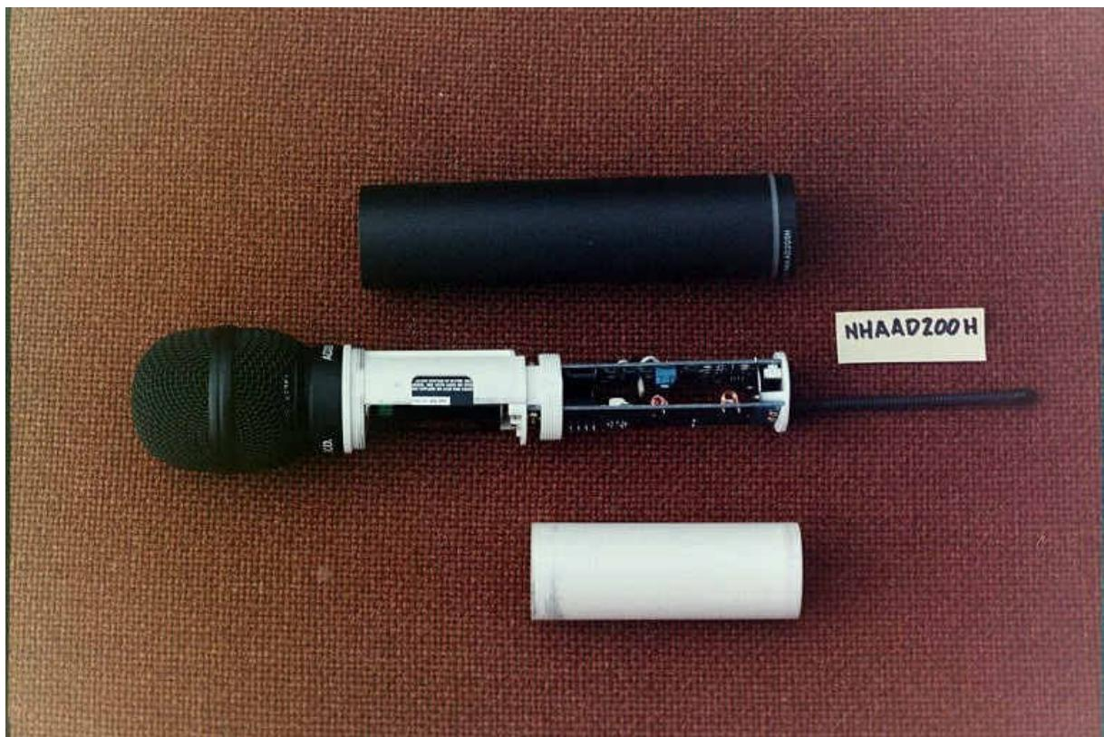
**FIGURE 40: Microphone Transmitter w/ Sleeves Removed B**
