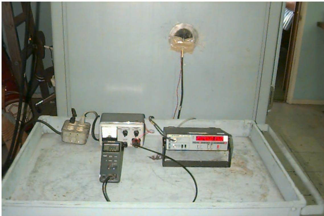
**FIGURE 34: Photograph of Frequency Stability Test Setup**
