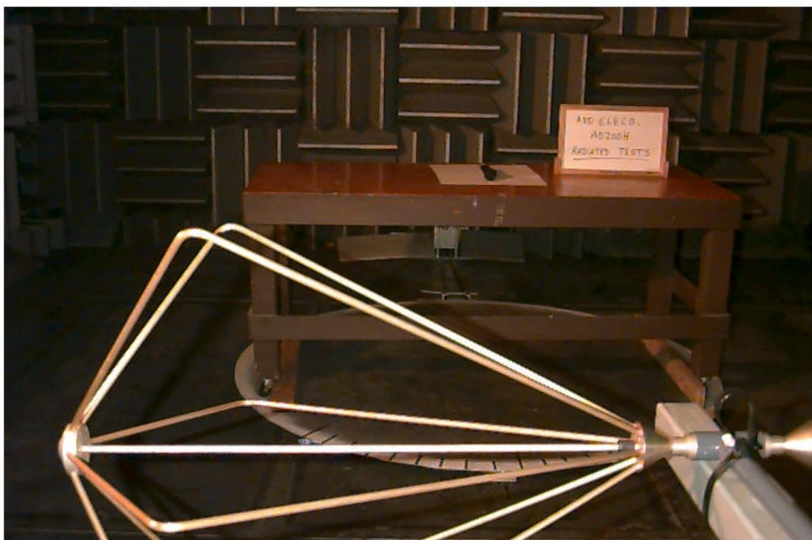
**FIGURE 23: Photograph of Radiated Spurious Emission Setup**
