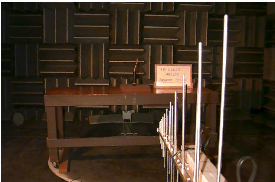
**FIGURE 24: Photograph of Radiated Spurious Emission Setup**
