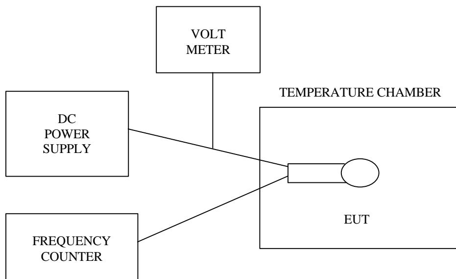
**FIGURE 33: Photograph of Frequency Stability Test Setup**
