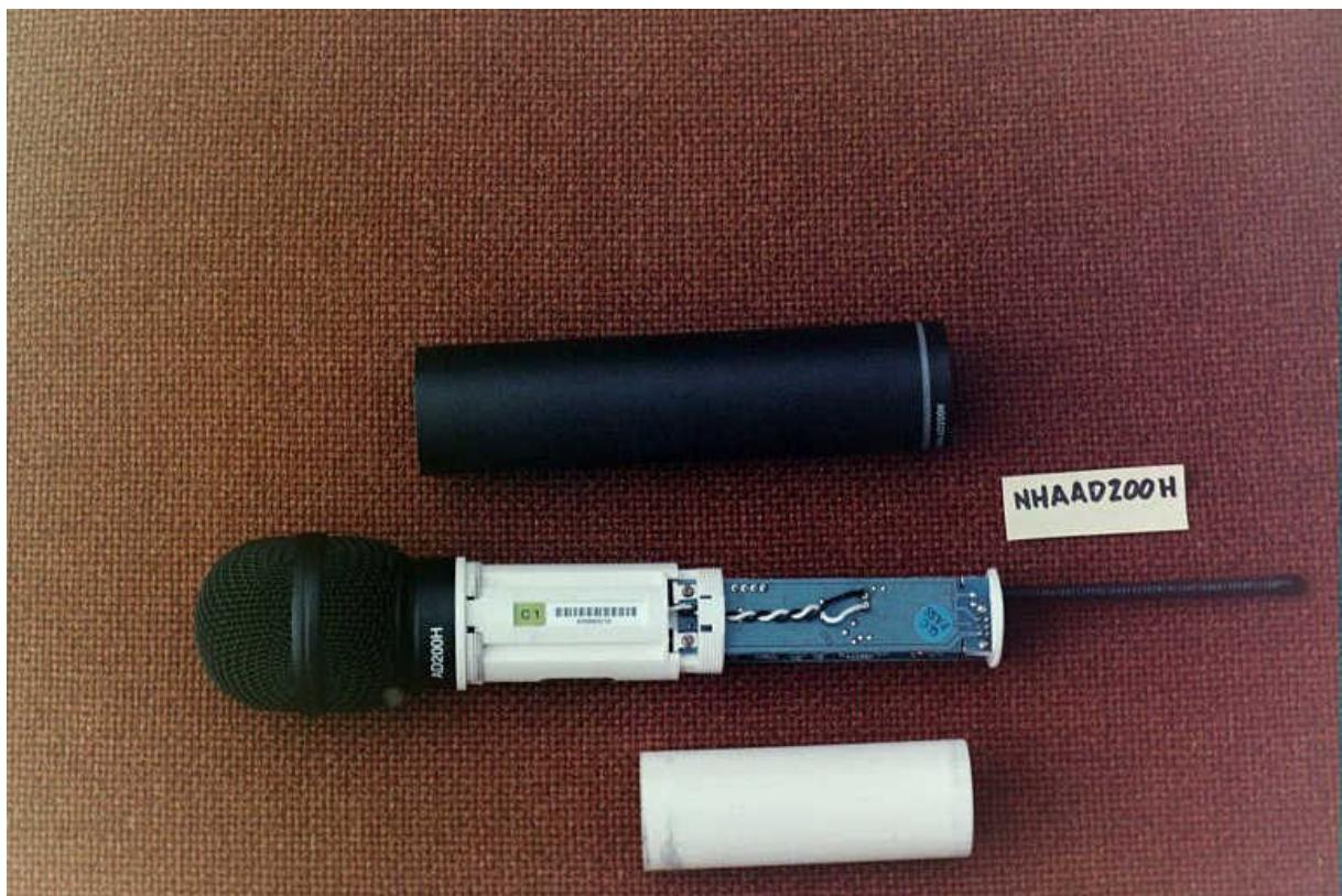
**FIGURE 41: Microphone Transmitter w/ Sleeves Removed C**
