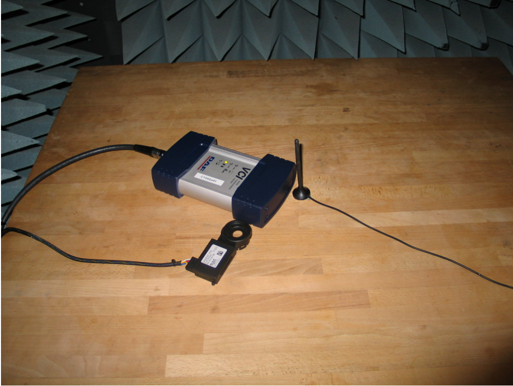
PHOTO No. 1: Setup for radiated measurements below 30 MHz
