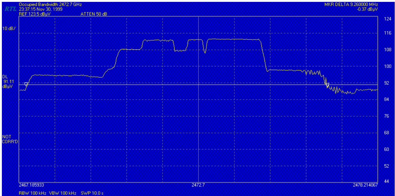
FIGURE 4: BANDWIDTH DETERMINATION 9.26 MHZ
