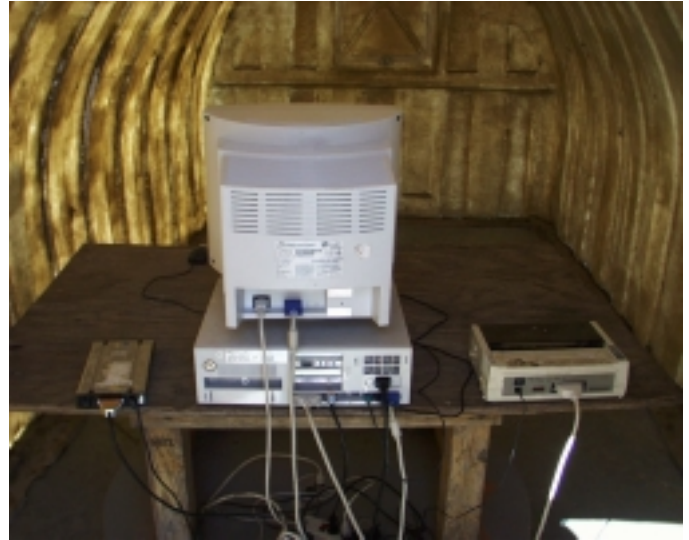
Radiated Emission Setup Photos (Worst Emission Position)
