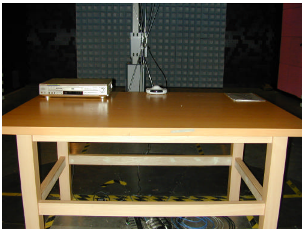
Back View of Radiated Test
