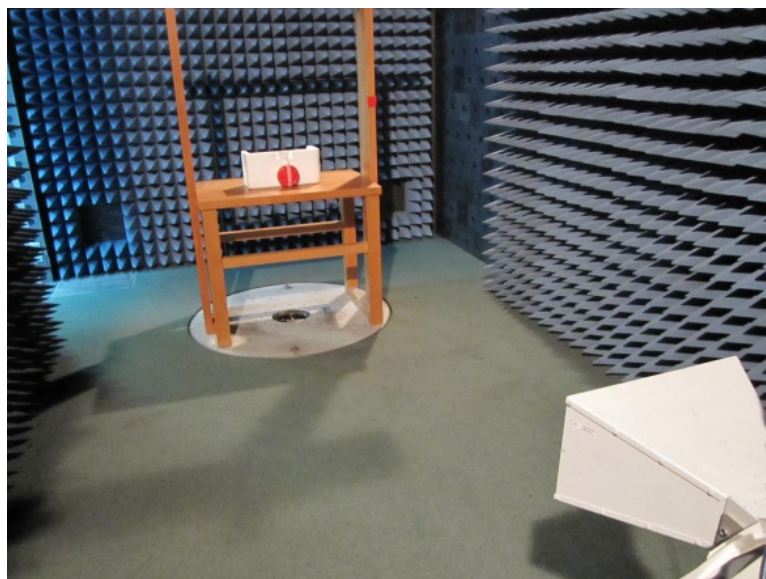
Photograph 8.1.3 Setup for radiated emission measurements
