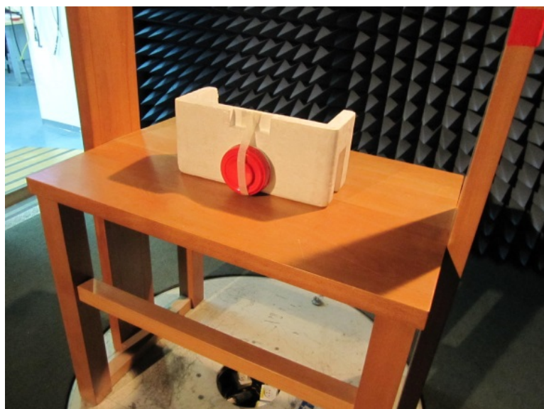
Photograph 8.1.3 Setup for radiated emission measurements
