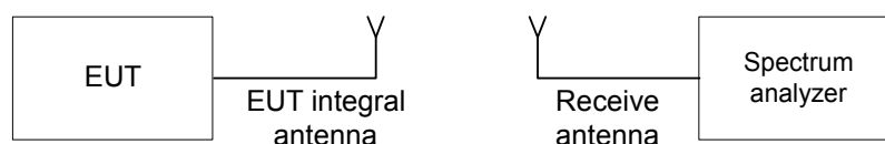
Figure 7.1.1 Setup for transmitter shut down test
