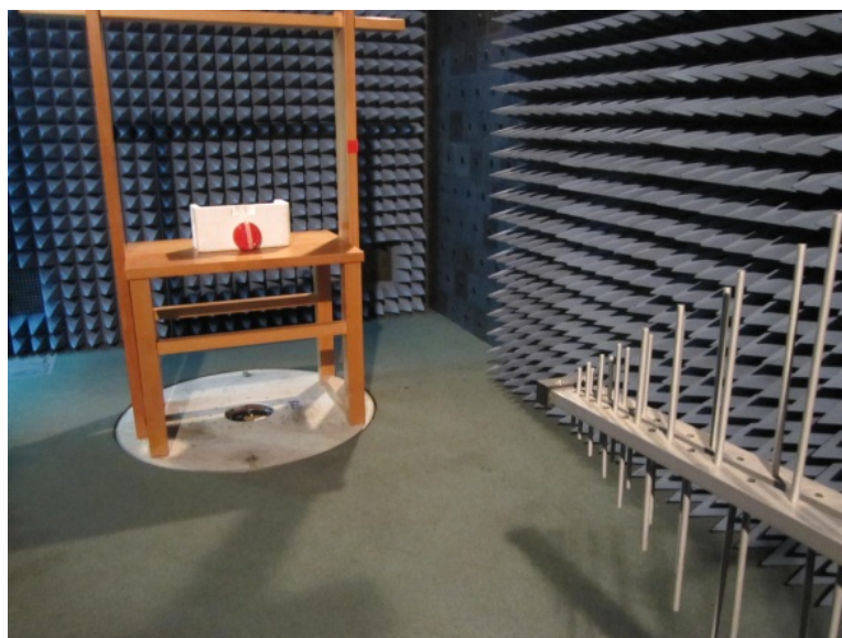
Photograph 8.1.1 Setup for radiated emission measurements
