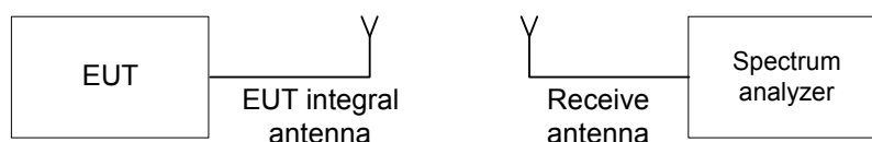
Figure 7.1.1 Setup for transmitter shut down test
