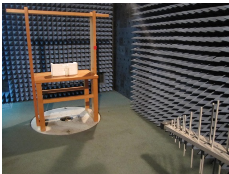
Photograph 8.1.1 Setup for radiated emission measurements
