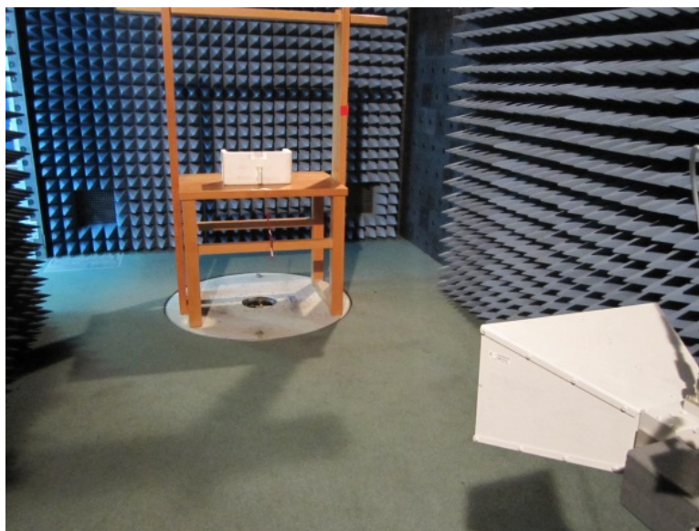
Photograph 8.1.3 Setup for radiated emission measurements
