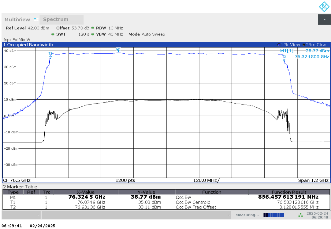
Plot no. 18: 99% OBW, Peak detector, -20 °C, DMP01
