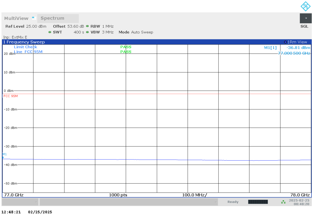
Plot no. 57: radiated emissions 77 GHz – 78 GHz, polarization vertical / horizontal, DMP01
