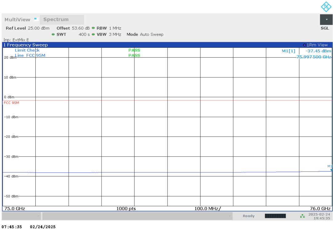
Plot no. 70: radiated emissions 75 GHz – 76GHz, band edge, DMP02
