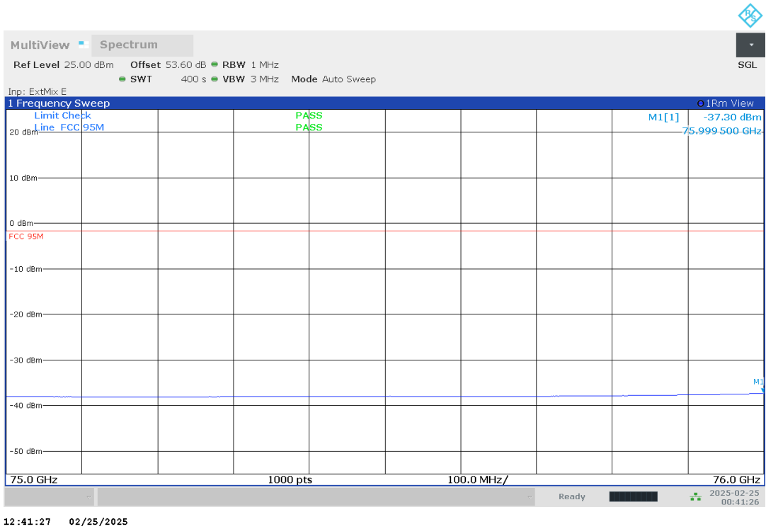
Plot no. 56: radiated emissions 75.0 GHz – 76.0 GHz, band edge, DMP01
