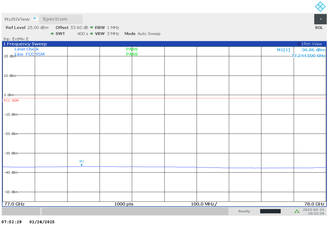
Plot no. 71: radiated emissions 77 GHz – 78 GHz, polarization vertical / horizontal, DMP02
