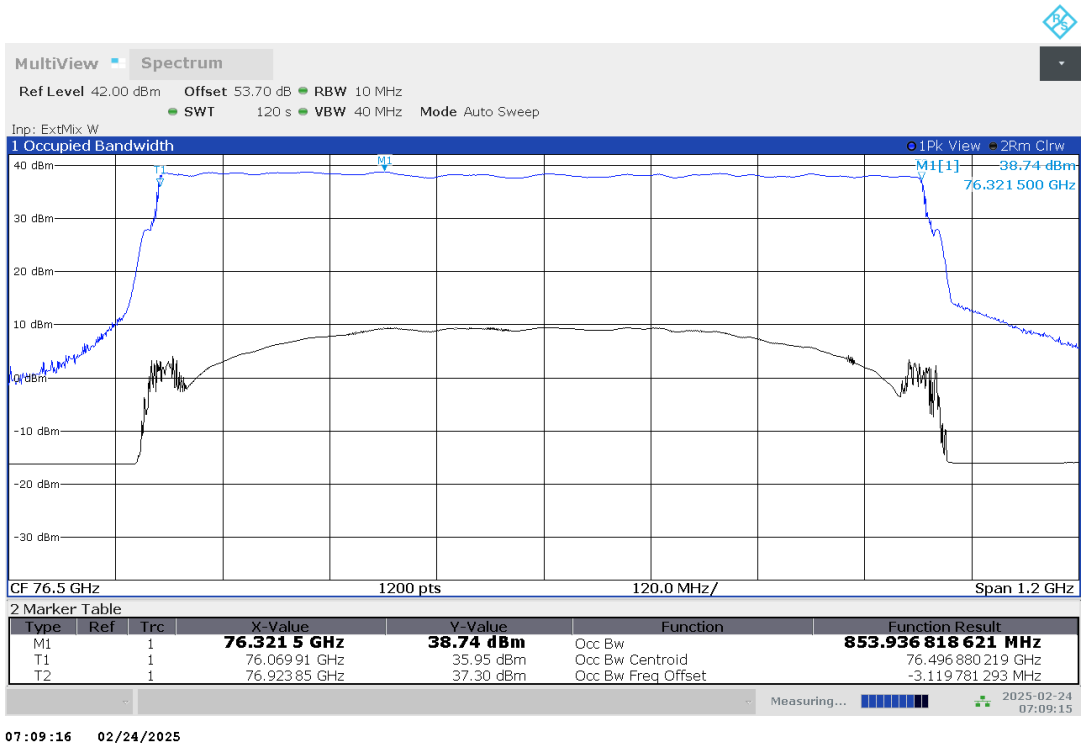
Plot no. 8: 99% OBW, Peak detector, 60 °C, DMP01
