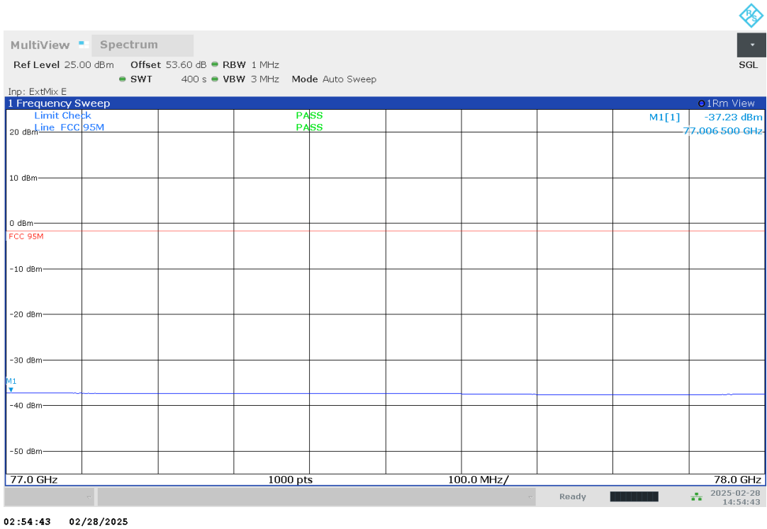
Plot no. 85: radiated emissions 77 GHz – 78 GHz, polarization vertical / horizontal, DMP03
