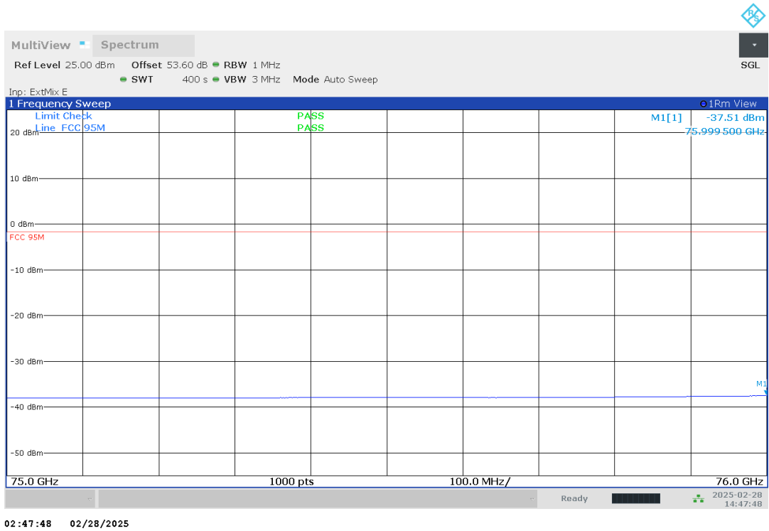
Plot no. 84: radiated emissions 75 GHz – 76 GHz, band edge, DMP03
