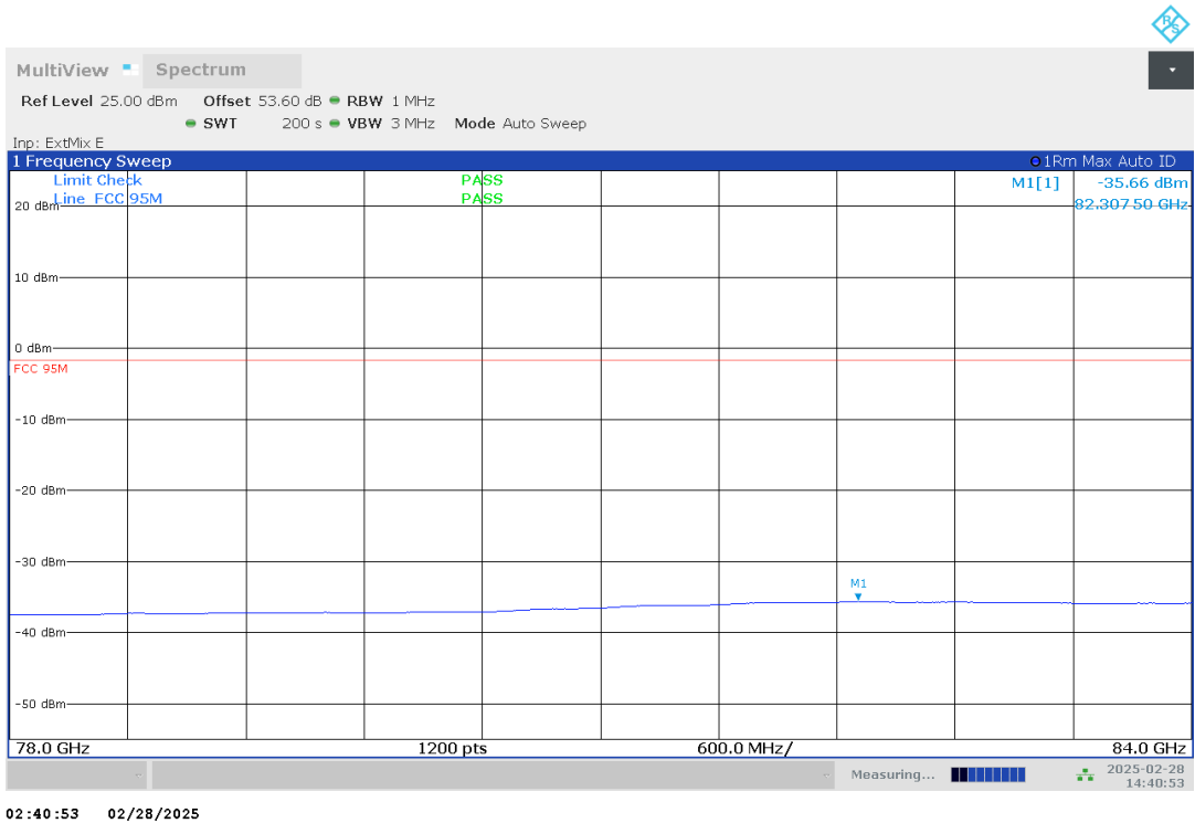
Plot no. 86: radiated emissions 78 GHz – 84 GHz, polarization vertical / horizontal, DMP03
