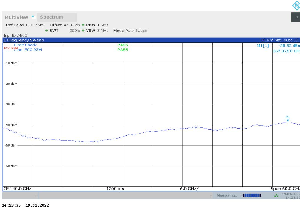
Plot no. 82: radiated emissions 170 GHz – 220 GHz, mode 6, polarization vertical / horizontal
