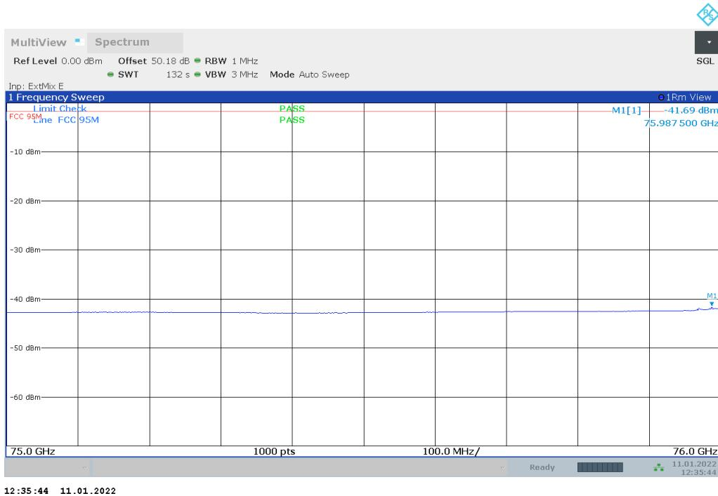
Plot no. 72: radiated emissions Band Edge High, mode 12, polarization vertical / horizontal
