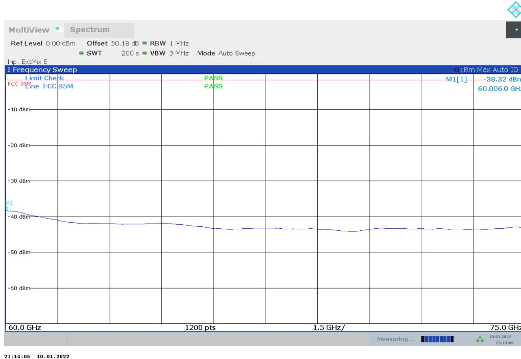
Plot no. 66: radiated emissions 60 GHz – 75 GHz, mode 12, polarization vertical / horizontal
