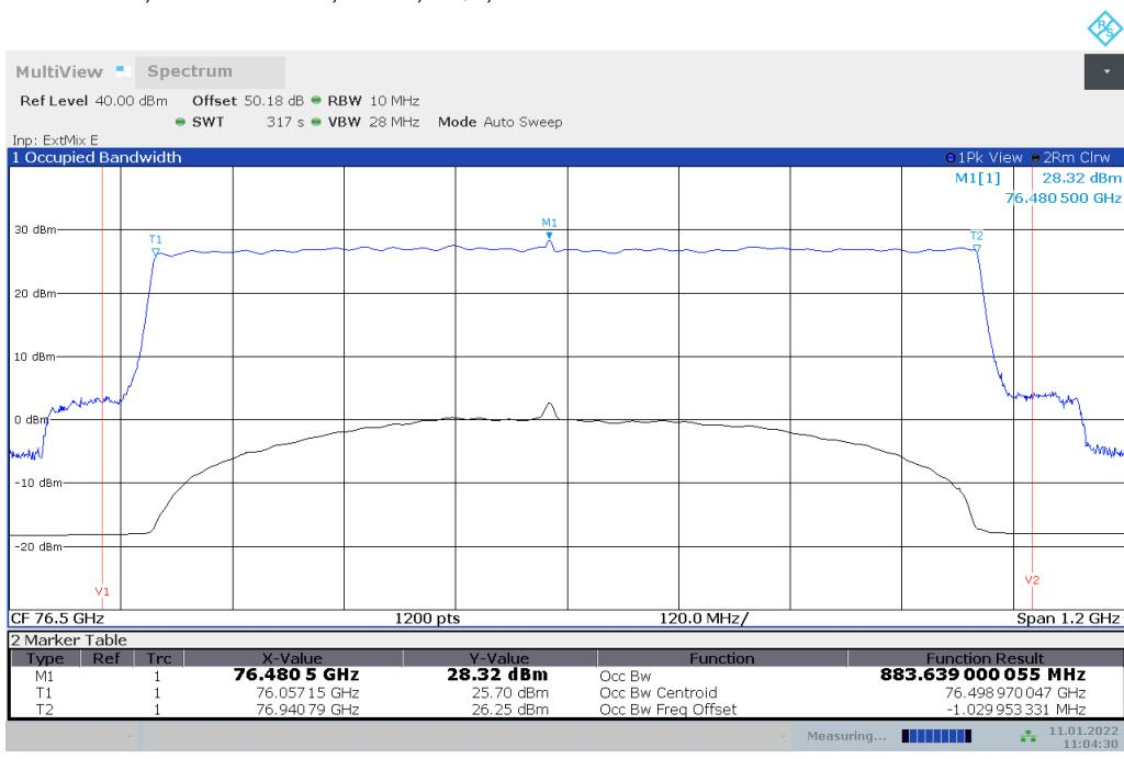
Plot no. 39: 99% OBW, Peak detector, 20 °C, V<sub>max</sub>, Test mode 12
