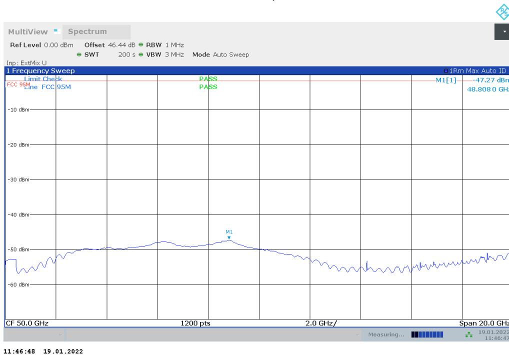
Plot no. 63: radiated emissions 40 GHz – 60 GHz, mode 12, polarization vertical / horizontal
