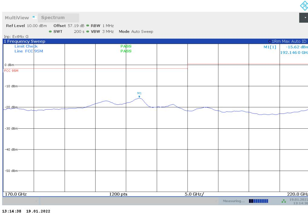
Plot no. 84: radiated emissions 170 GHz – 220 GHz, mode 12, polarization vertical / horizontal
