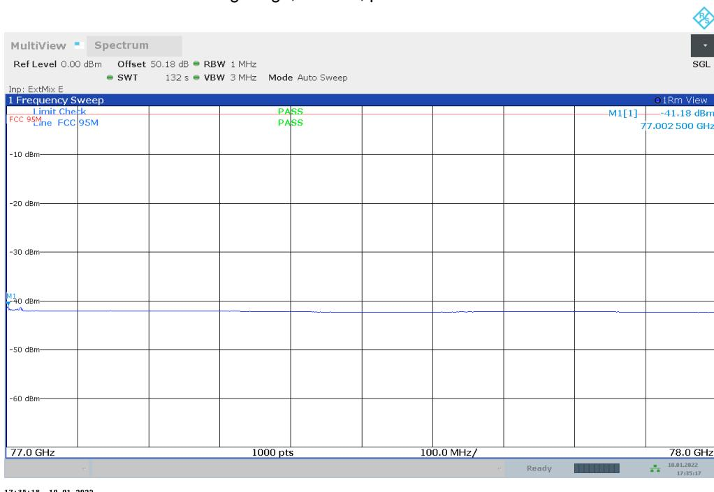
Plot no. 69: radiated emissions Band Edge Low, mode 8, polarization vertical / horizontal
