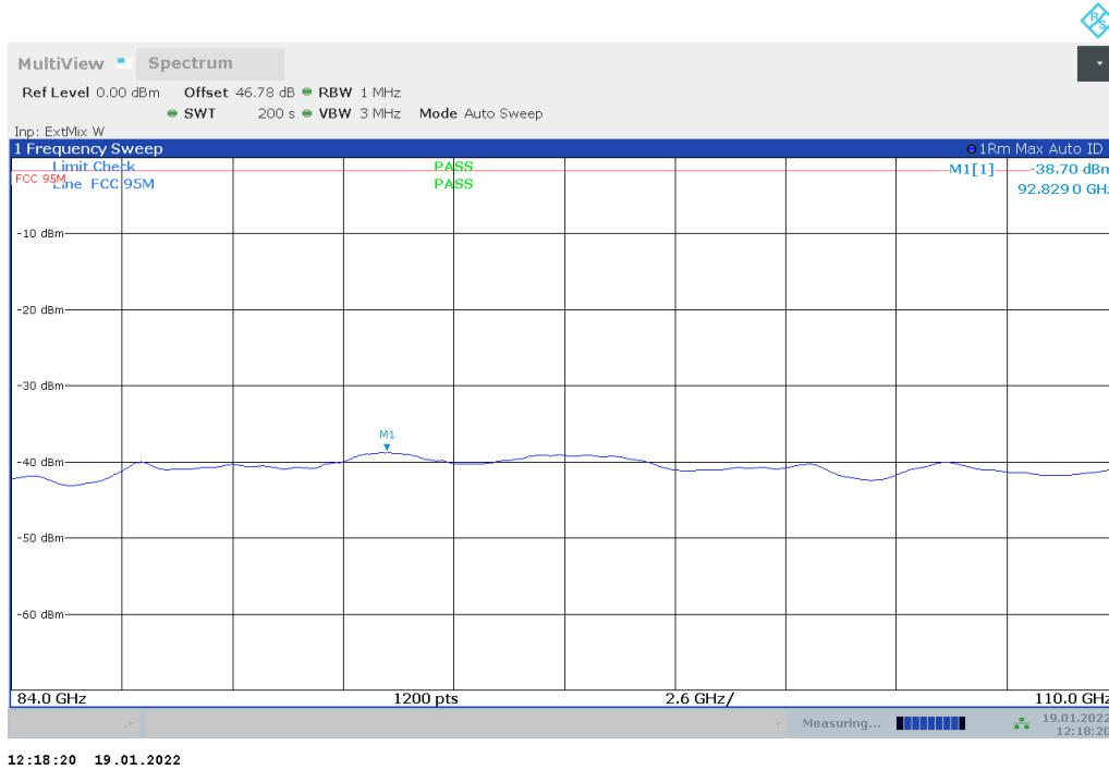
Plot no. 78: radiated emissions 84 GHz – 110 GHz, mode 12, polarization vertical / horizontal
