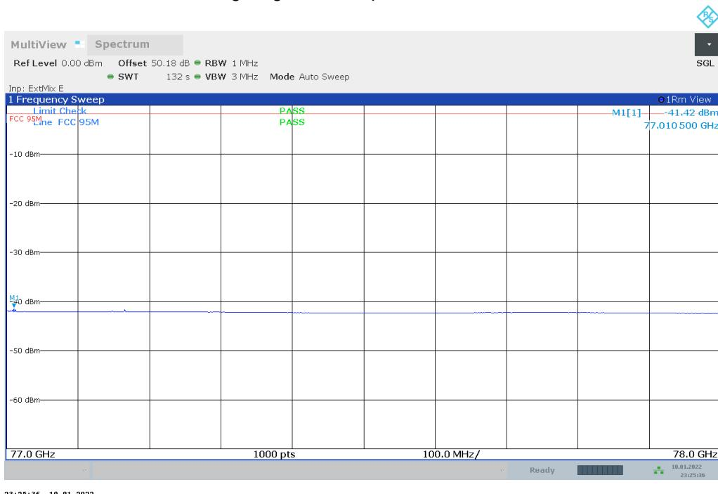
Plot no. 71: radiated emissions Band Edge Low, mode 12, polarization vertical / horizontal
