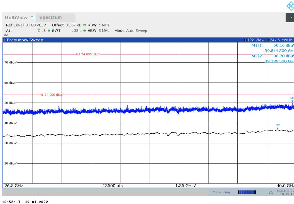
Plot no. 60: radiated emissions 26.5 GHz – 40 GHz, mode 12, polarization vertical / horizontal
