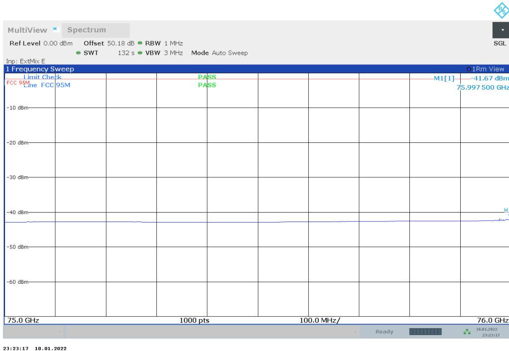
Plot no. 70: radiated emissions Band Edge High, mode 8, polarization vertical / horizontal
