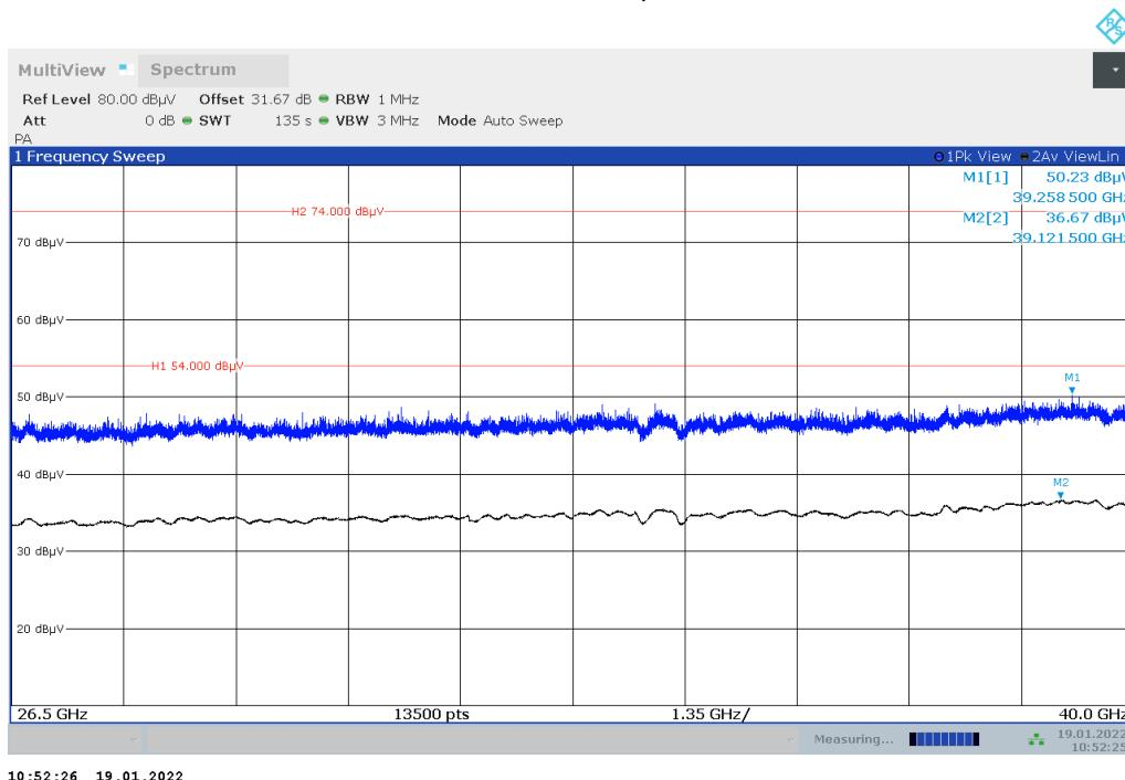
Plot no. 61: radiated emissions 40 GHz – 60 GHz, mode 6, polarization vertical / horizontal
