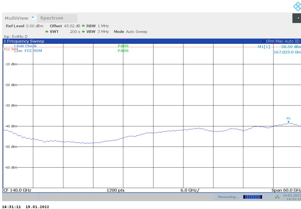
Plot no. 81: radiated emissions 110 GHz – 170 GHz, mode 12, polarization vertical / horizontal
