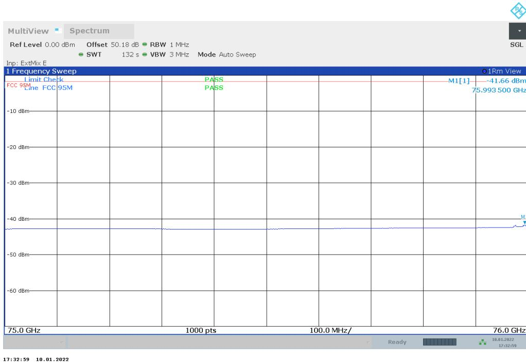
Plot no. 68: radiated emissions Band Edge High, mode 6, polarization vertical / horizontal
