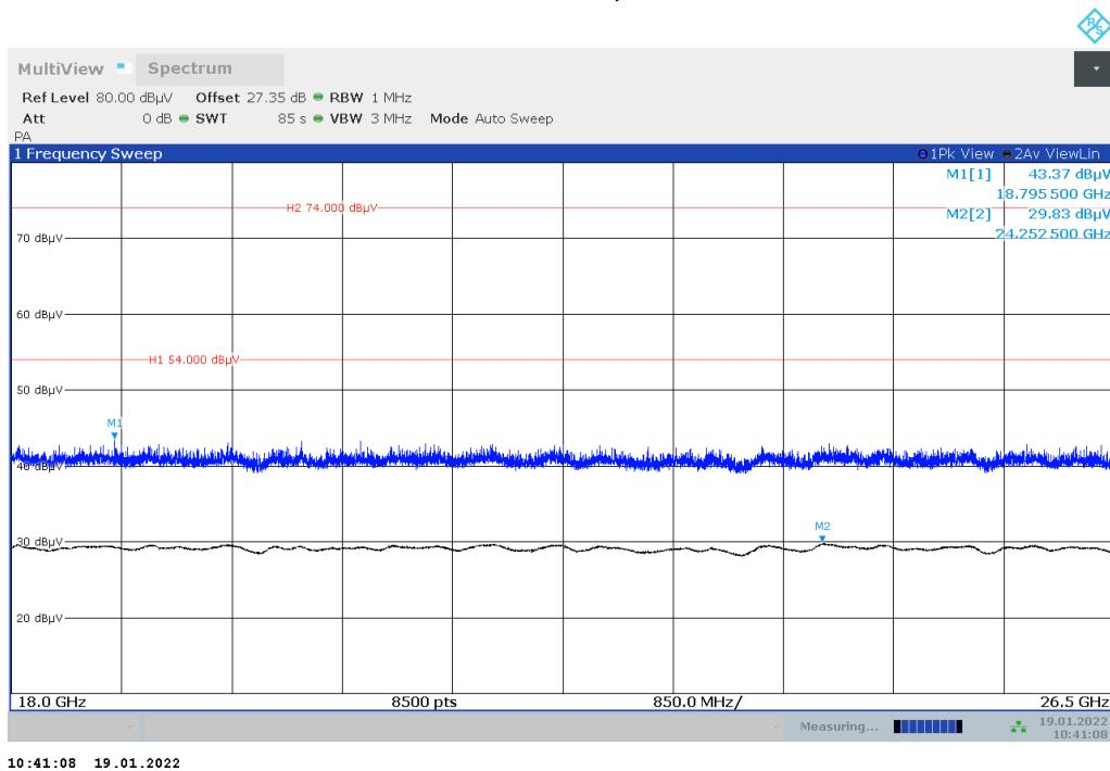
Plot no. 57: radiated emissions 18 GHz – 26.5 GHz, mode 12, polarization vertical / horizontal
