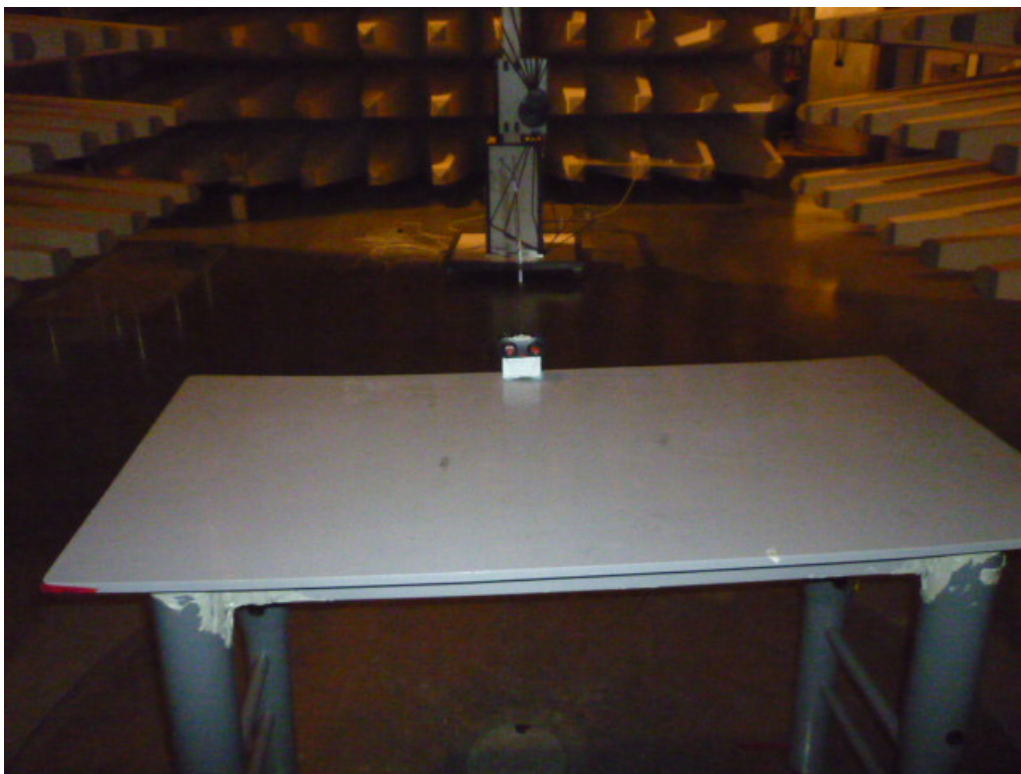
Set-up for Radiated Emission (Transmitter)
