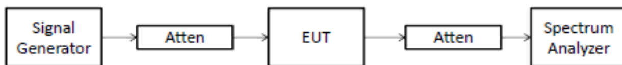
Figure 7.7.1 Spurious emission test setup
