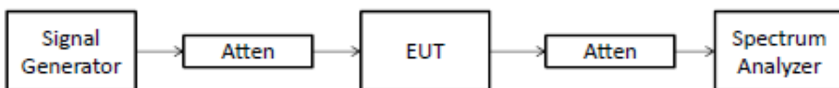
Figure 7.4.1 Emission mask test setup
