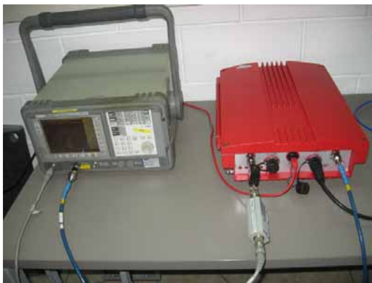
Photograph 7.8.1 Noise figure test setup
