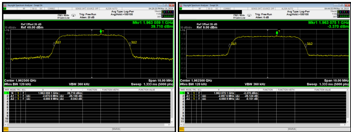
Plot 3.2.3: Input-versus-output signal comparison, AWGN 4.1MHz, 0.5 dB below AGC threshold level
