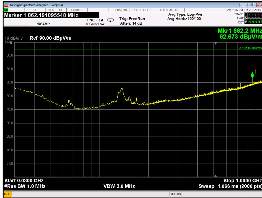
Plot 3.6.1: Spurious Emission test results, 30 MHz – 1 GHz range, Horizontal polarization, Low Frequency
