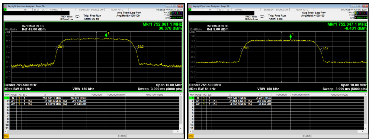
Plot 3.2.2: Input-versus-output signal comparison, AWGN 4.1MHz, 3 dB above AGC threshold level
