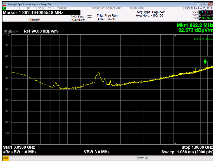
Plot 3.6.2: Spurious Emission test results, 30 MHz – 1 GHz range, Vertical polarization, Low Frequency
