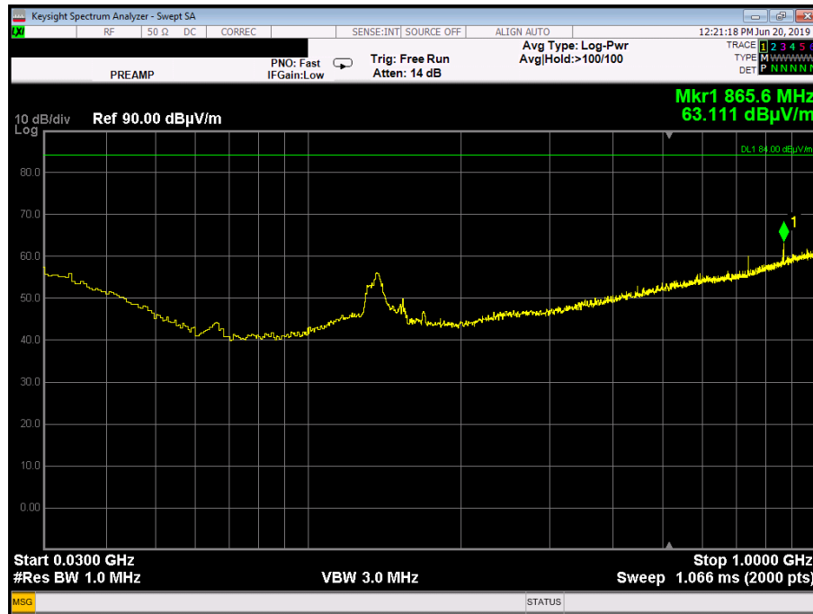
Plot 3.6.6: Spurious Emissions test results, 30 MHz – 1 GHz range, Vertical polarization, Middle Frequency
