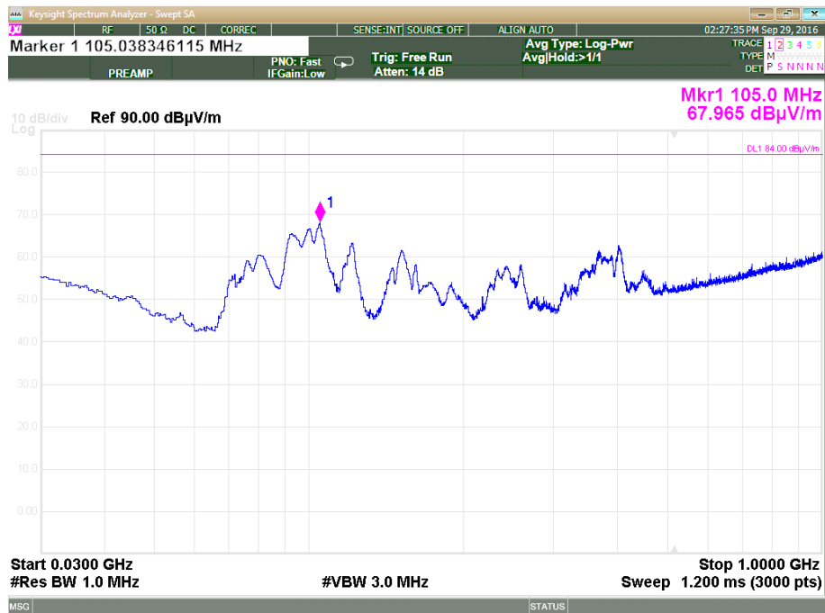
Plot 3.6.14: Spurious Emissions test results, 30 MHz – 1 GHz range, Vertical polarization, Low Frequency
