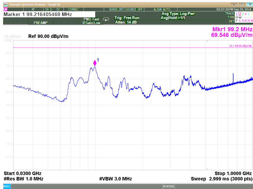
Plot 3.6.18: Spurious Emissions test results, 30 MHz – 1 GHz range, Vertical polarization, Middle Frequency
