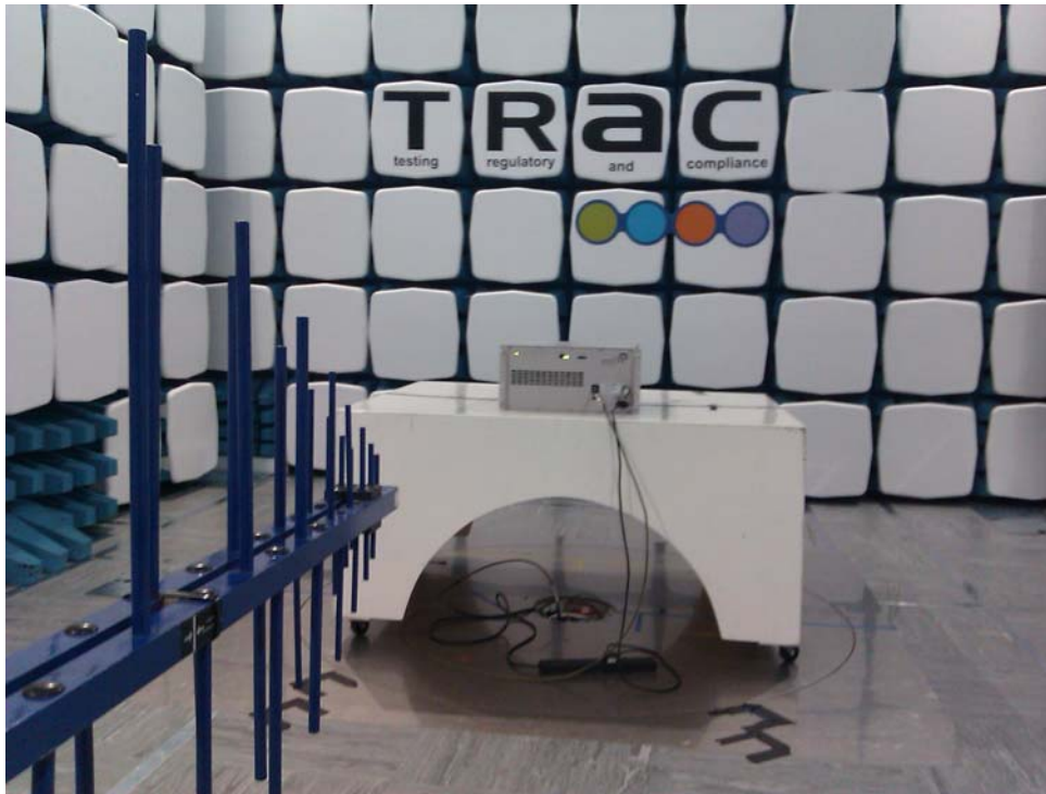
Photograph 1: Setup for radiated tests
