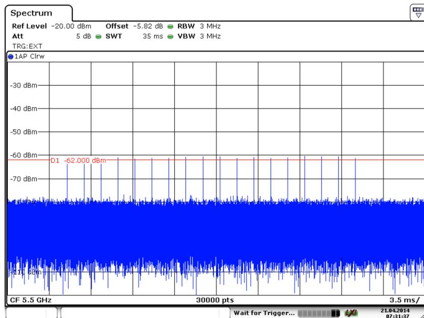
**<40MHz / 5510 MHz> Radar Type 1****Radar / DFS detection threshold level and the burst of pulses on the Channel frequency**
