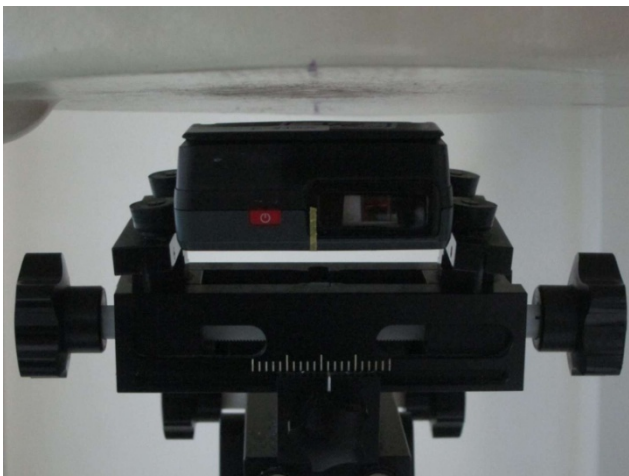
Back of the DUT with Phantom 1 cm Gap for sample 4
