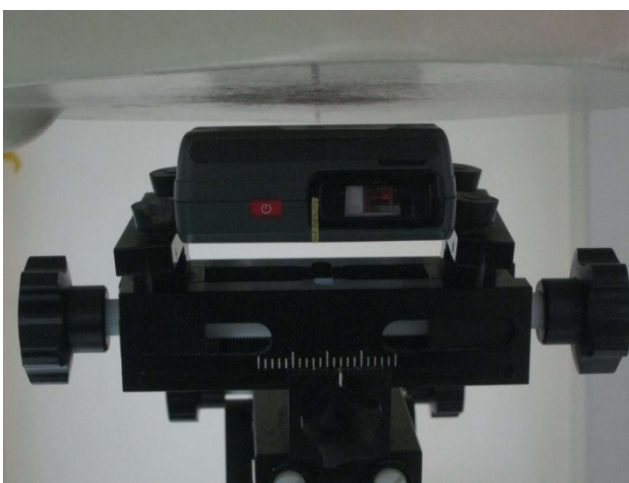
Back of the DUT with Phantom 1 cm Gap for sample 3
