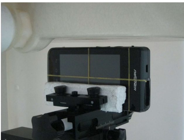
Left Side of the DUT with Phantom 1 cm Gap for sample 1
