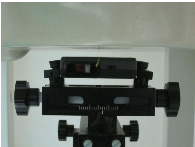
Front of the DUT with Phantom 1 cm Gap for sample 1
