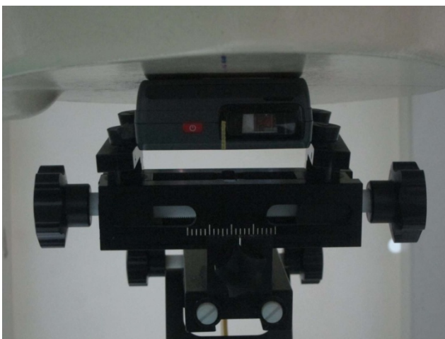
Back of the DUT with Phantom 0 cm Gap with earphone for sample 3
