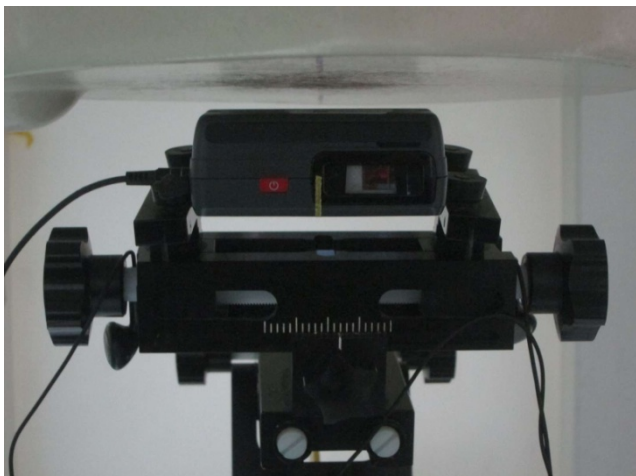
Back of the DUT with Phantom 1 cm Gap with earphone for sample 3
