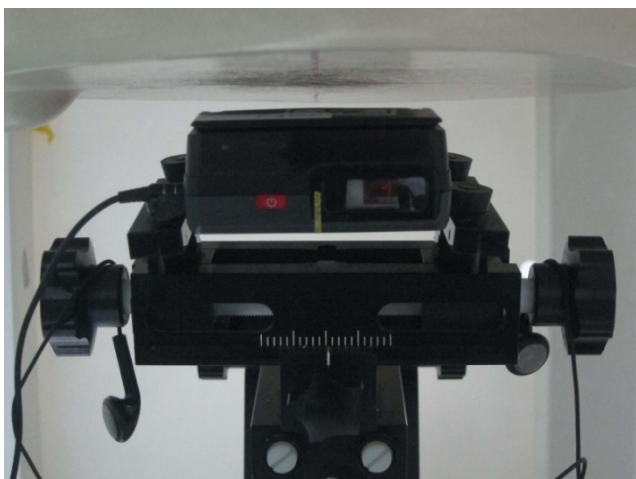
Back of the DUT with Phantom 1 cm Gap with earphone for sample 4
