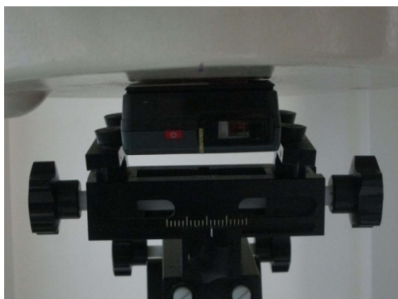
Back of the DUT with Phantom 0 cm Gap with earphone for sample 4
