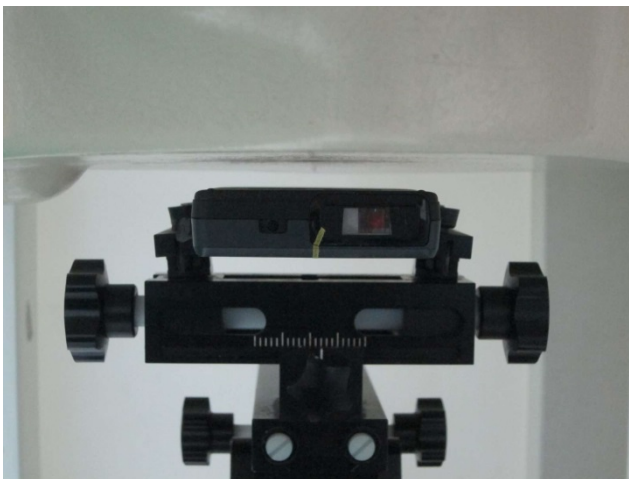
Back of the DUT with Phantom 1 cm Gap for sample 1
