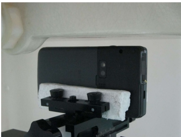
Right Side of the DUT with Phantom 1 cm Gap for sample 1
