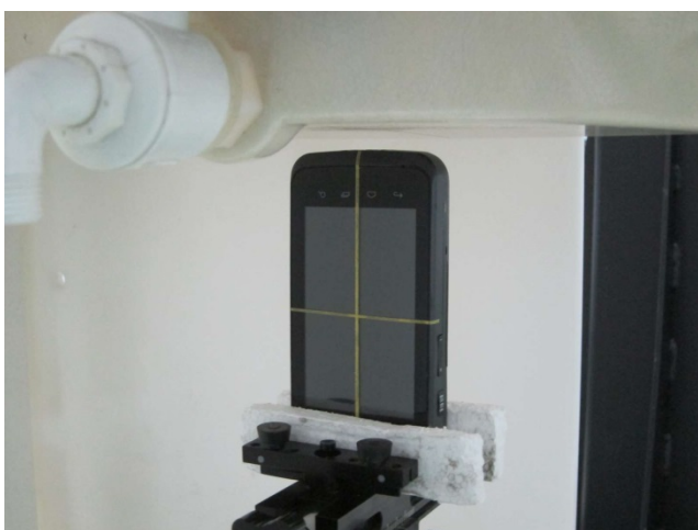
Bottom Side of the DUT with Phantom 1 cm Gap for sample 1
