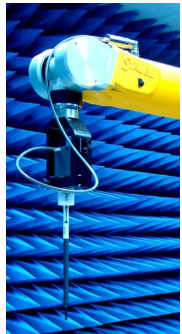
Figure 4. Probe setup on robot
