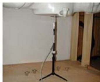
Figure 12.1 Dipole Validation Test Setup
