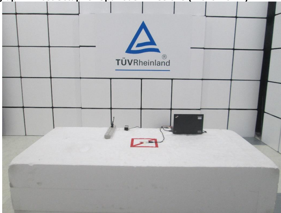
Photograph 2: Test Setup for Spurious Emissions (Front View 2)
