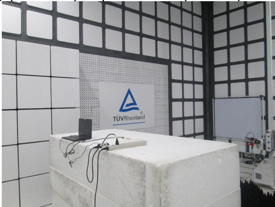
Photograph 6: Test Setup for Spurious Emissions (Back View 4)
