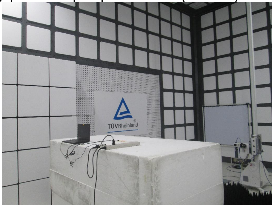
Photograph 6: Test Setup for Spurious Emissions (Back View 4)
