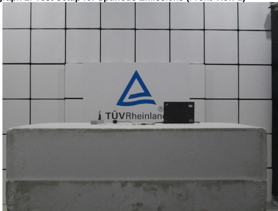
Photograph 2: Test Setup for Spurious Emissions (Front View 2)
