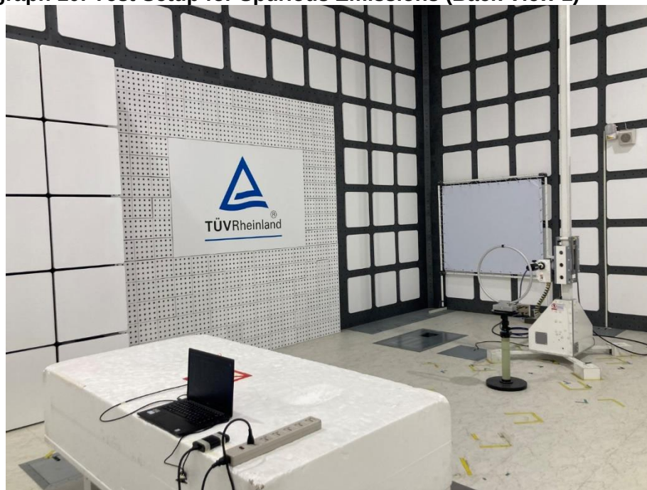
Photograph 10: Test Setup for Spurious Emissions (Back View 1)
