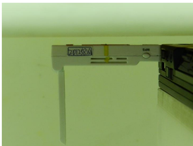
Horizontal Up with Phantom 5 mm Gap Antenna swivel 90 degree
