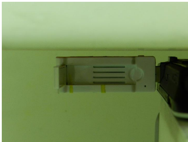
Vertical Front with Phantom 5 mm Gap Antenna swivel 90 degree
