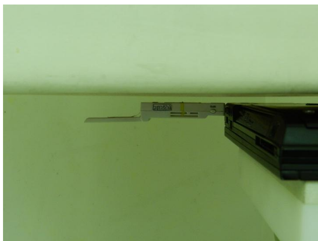
Horizontal Up with Phantom 5 mm Gap Antenna swivel 180 degree
