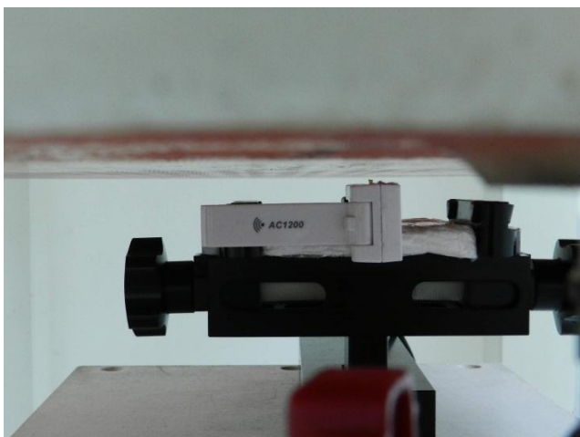
Vertical Back with Phantom 5 mm Gap Antenna swivel 90 degree
