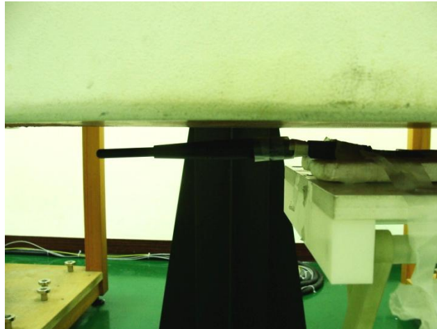
USB Cable Plug-in for USB Configuration 2 (USB Horizontal Down with Phantom 5 mm Gap, Antenna in Straight Mode)
