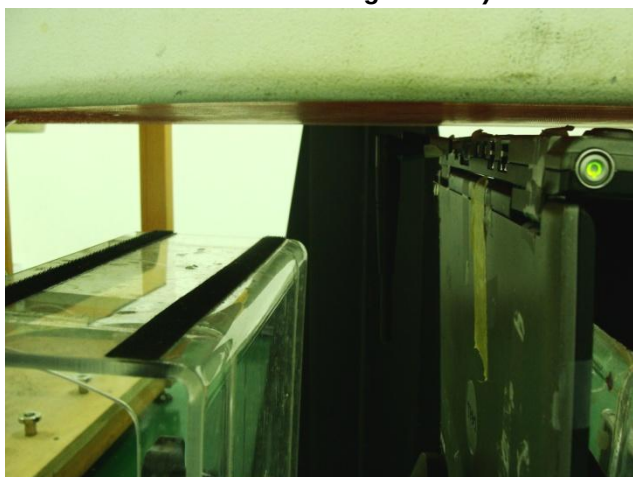
Direct Laptop Plug-in for USB Configuration 1 (USB Horizontal Up with Phantom 5 mm Gap, Antenna in Vertical Mode)
